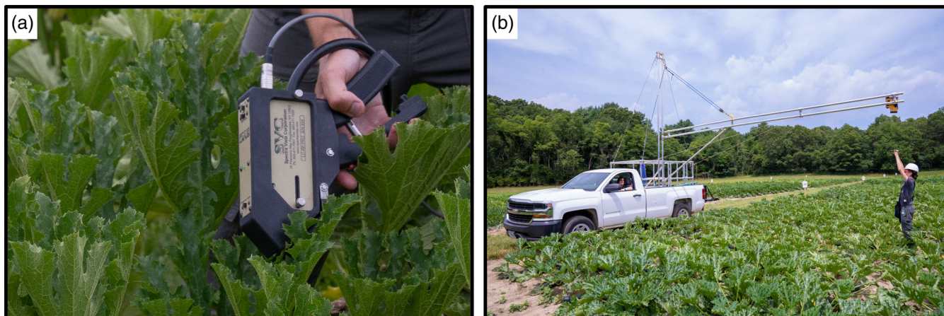
FIGURE 4 Photographs show spectral data collection at leaf (a) and canopy (b) levels. The spectroradiometer is referenced using a white Spectralon® disc for leaf-level measurements and a white Spectralon® plate for canopy-level measurements, shown in (b)
