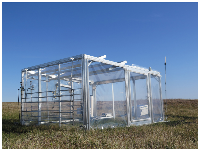
Figure 2. The ZPW chamber pictured on coastal tundra near Barrow, AK. The chamber measures 2.4\text{ m} \times 2.4\text{ m} \times 1.4\text{ m} ( L \times W \times \text{maximum } H ). In this picture, the two vents are partially open due to the temperature differential between the internal and external heat exchangers that are visible on the near wall of the chamber. The brass pistons and counterweight (section of white PVC pipe) can be seen opposite the door. The near corner obscures the view of most of the monitoring instrumentation but the junction box can be seen in the centre of the far wall. Outside and behind the chamber you can see a box with a solar panel that contains a data logger and battery to power the monitoring instrumentation, and an antenna for data communication.
