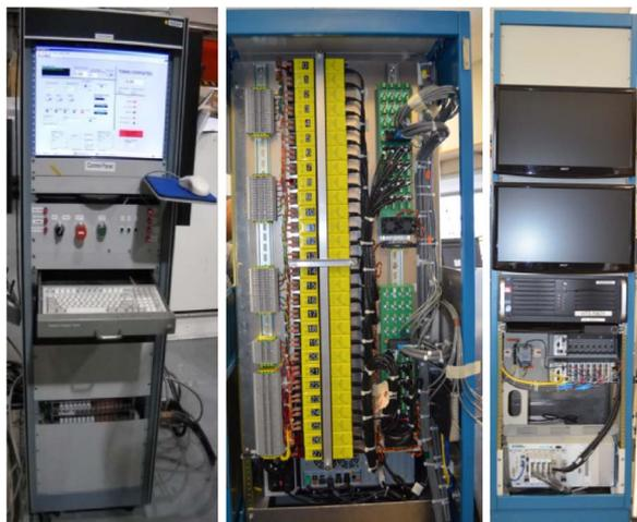
Fig. 11. Part of the advanced quench detection electronics system that was specifically developed to have a high sensitivity to detect the onset of the prequench phase at the millivolts or lower level in large coils and tolerate high isolation voltage (over 1 kV) for fast energy extraction.
