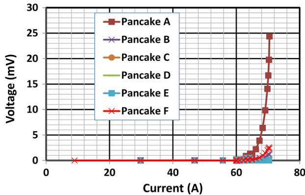
Fig. 10. Measured performance ( $V-I$  curve) at 77 K (in liquid nitrogen) of individual pancake coils when all six are powered together in series.
