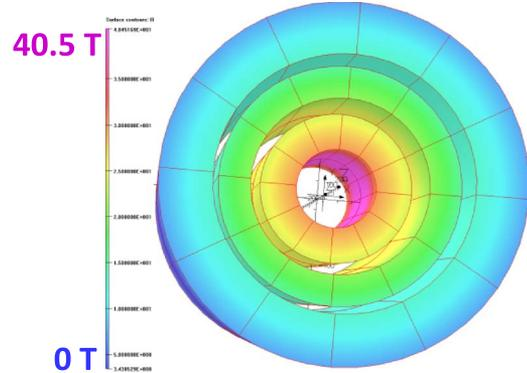
Fig. 13. Magnetic design of a hybrid  $\sim 40\text{-T}$  solenoid. Two inner coils are made with HTS, and the outer coil is made with LTS.
