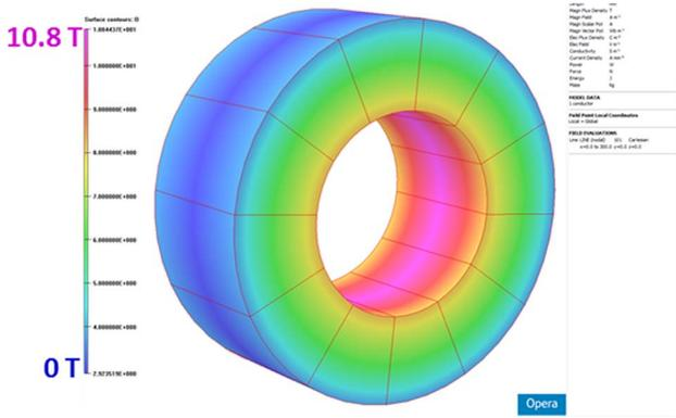
Fig. 1. Computed field contour on the surface of the conductor in the 100-mm-aperture six pancake HTS solenoid built and tested at 590 A.
