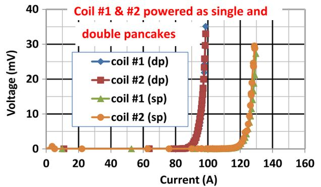
Fig. 7. Measured performance ( $V-I$  curve) at 77 K (in liquid nitrogen) of pancake coils #1 and #2 when powered in single-pancake (individually) and double-pancake (together) configurations.
