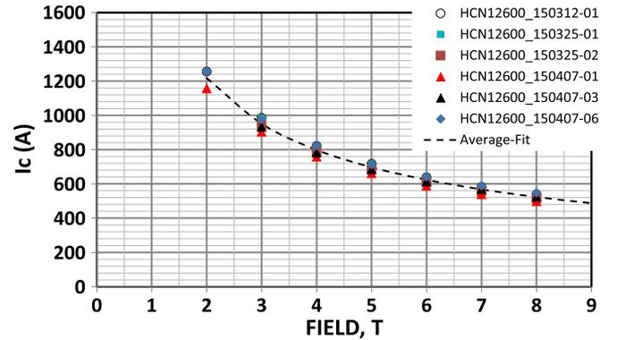
Fig. 3. Critical current at 4.2 K versus field applied perpendicular to the wide face of the tape. The variation between the six samples is quite small.
