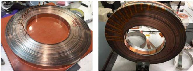
Fig. 5. (Left) Single-pancake coil with voltage taps. (Right) Double-pancake unit made with two single pancakes with a spiral splice joint inside.
