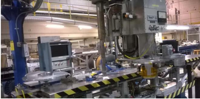
Fig. 4. Computer-controlled automatic winder used for winding CAPP coils.
