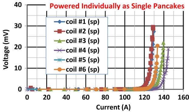
Fig. 8. Measured performance of pancake coils #1 through #6 at 77 K when powered in single-pancake configuration.
