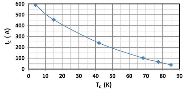
Fig. 12. Critical current as a function of critical temperature for the criterion of  $\sim 1.5 \text{ mV}$  over or  $0.1 \mu\text{V}/\text{cm}$  over the entire CAPP/IBS solenoid.
