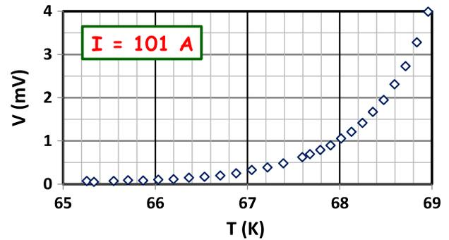
Fig. 11. Measurement of critical temperature of CAPP/IBS solenoid at  $\sim 101 \text{ A}$  when the current is held constant and coil is allowed to warm up slowly. The criterion of  $1.5 \text{ mV}$  or  $0.1 \mu\text{V}/\text{cm}$  implies a critical temperature of  $\sim 68.3 \text{ K}$ .
