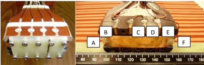
Fig. 2. Sample layout of the BNL test holder. The voltage taps at locations A through F are indicated.
