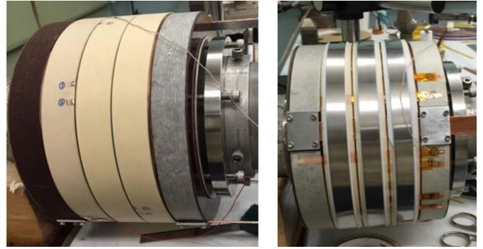
Fig. 6. (Left) Fiberglass epoxy and (right) stainless steel band on each double-pancake unit as a part of the radial support structure.
