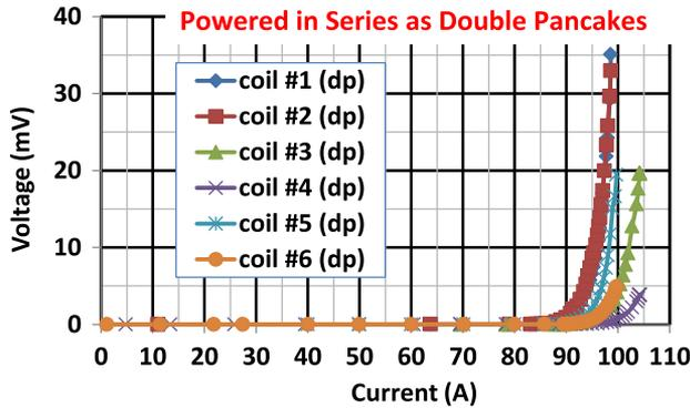
Fig. 9. Measured performance of pancake coils #1 through #6 at 77 K when powered in double-pancake configuration.
