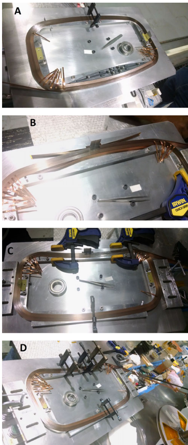
Fig. 2. Stages of the winding with HTS conductor. (a) Using filler piece to wind with positive curvature. (b) With filler piece removed. (c) Pushing inner side for negative curvature. (d) Clamping negative curvature side.
