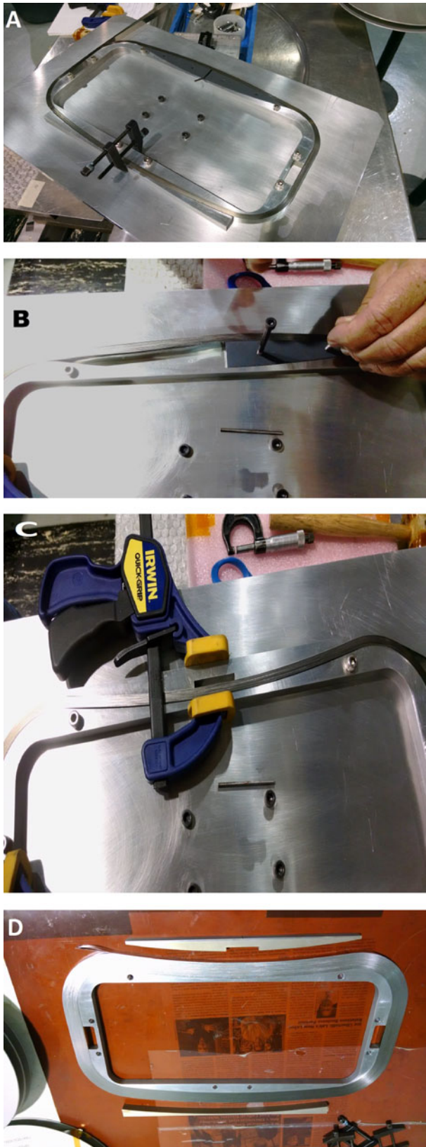
Fig. 1. Winding bobbin and tooling used for the practice wind with stainless steel tape. (a) Tape is wound with positive curvature on all sides of the bobbin using the special tooling. (b) The tooling is being removed before the practice coil is pressed into position on the negative curvature section. (c) The coil is clamped into place. (d) The completed practice coil with tooling used during winding is shown.
