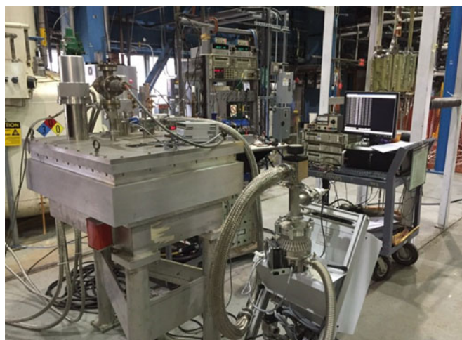
Fig. 10. Cryocooled magnet coils being tested.
