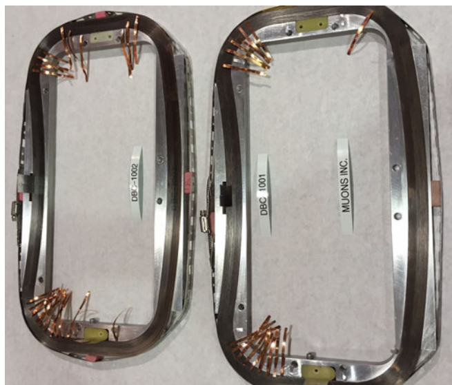
Fig. 3. Two single coil pancakes that will make up a double coil pancake.
