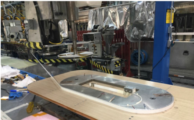
Fig. 3. Coil being wound with the universal coil winder with 4-ply ASC tape and Nomex insulation. A number of voltage-taps were also installed.
