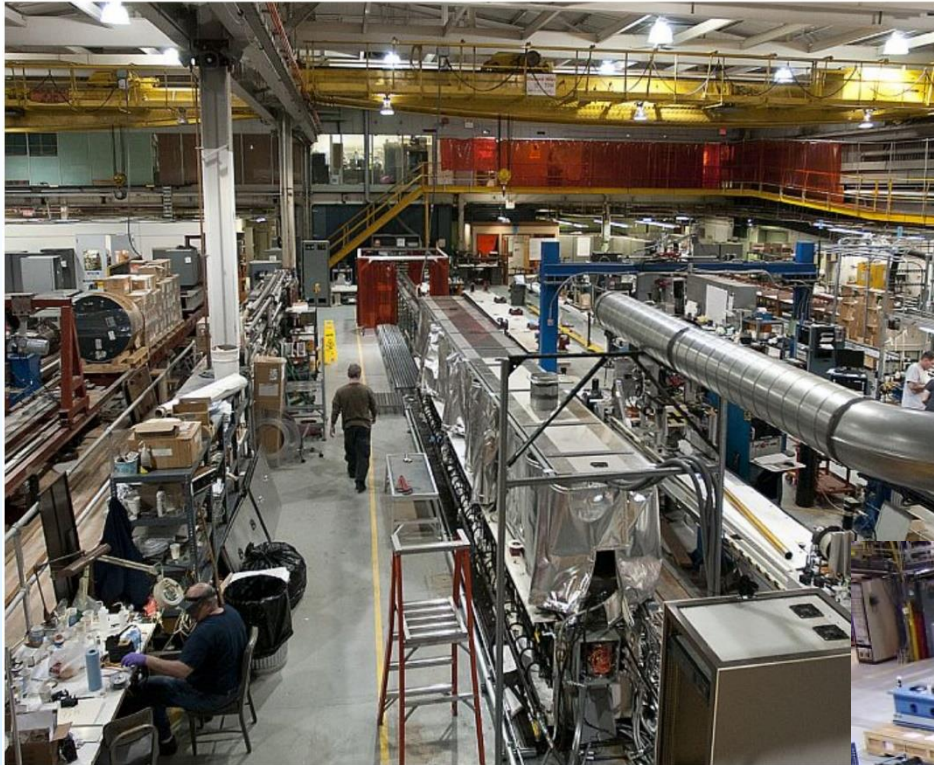
The coil, inserted in the form block, is heated electrically to set the epoxy that fixes the coil size. Heating is done inside an array of heavy copper (foreground) that minimizes heat loss.
