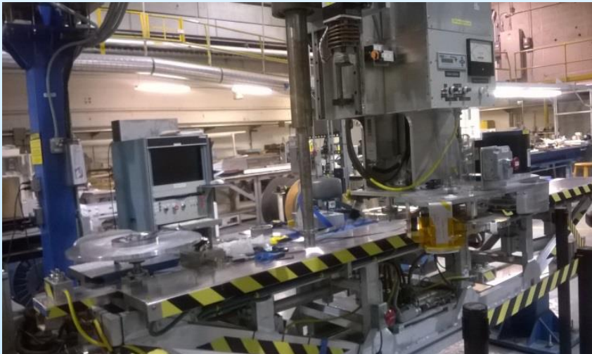
Semiautomatic coil winding with 10 m coil. The spool of cable used in the coil winding is in the foreground.
