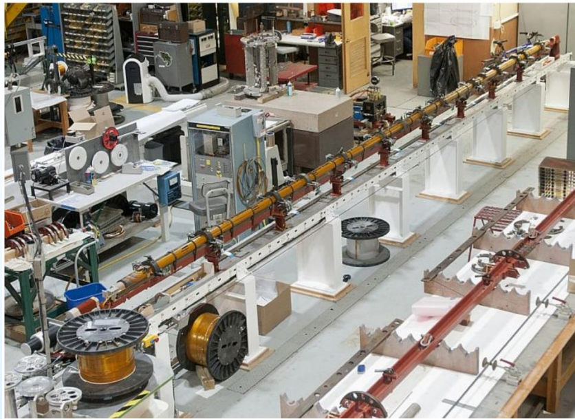
Semiautomatic coil winding with 10 m coil. The spool of cable used in the coil winding is in the foreground.
