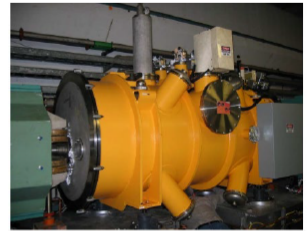
BNL AGS Snake Magnet (3 T max, 20 cm warm bore, LHe recondensing system)
