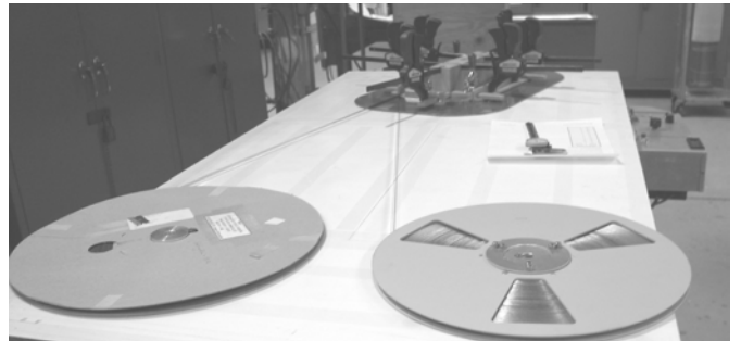
Fig. 6. A coil is being made by co-winding HTS tape (on right) and stainless steel insulating tape (left).
