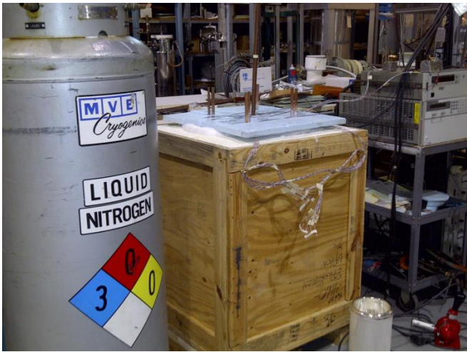
Fig. 9. A cryostat made of a stainless steel container installed inside a wooden frame, filled with insulating foam in between.
