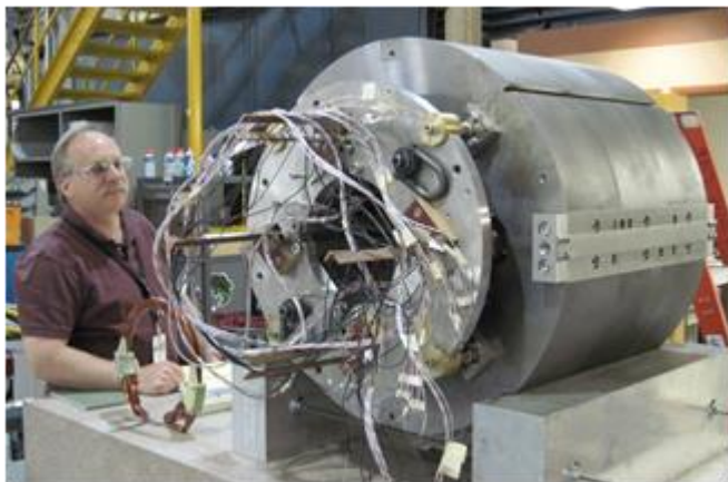
Fig. 6. Fully assembled FRIB quadrupole with support structure and iron yoke (cryostat for warm iron test is not yet installed).
