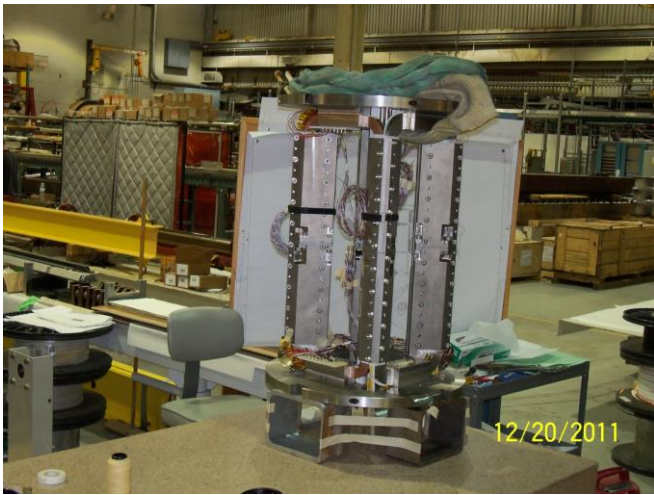
Fig. 5. Coils in support structure consisting of clamps and end plates.
