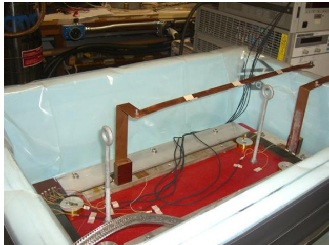
Fig. 8. Simple vessel made with Styrofoam for testing individual FRIB coils at 77 K in liquid nitrogen.
