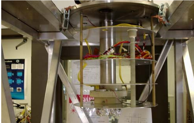
Fig. 5: HTS solenoid between the aluminum baffles. SRF Gun will be situated below this assembly.
