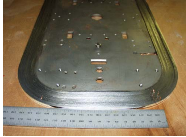
Fig. 7. FRIB R&D coil made with 2G HTS.
