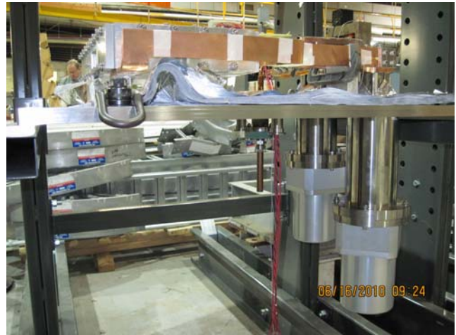
Fig. 9. A cryo-mechanical structure during fabrication that will test six 2G HTS coils. One can see two cryo-heads in the lower-right of the picture and coils in the bolted support structure on the upper-side.
