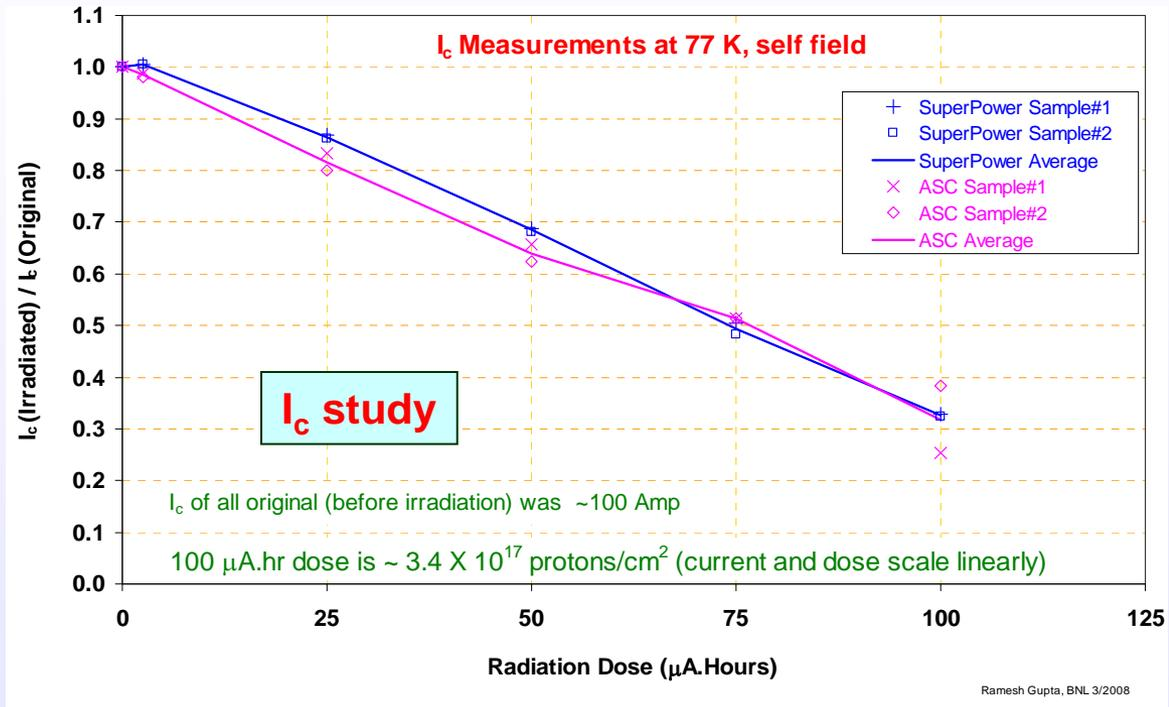
**Bottom line – YBCO is robust against radiation damage:**
