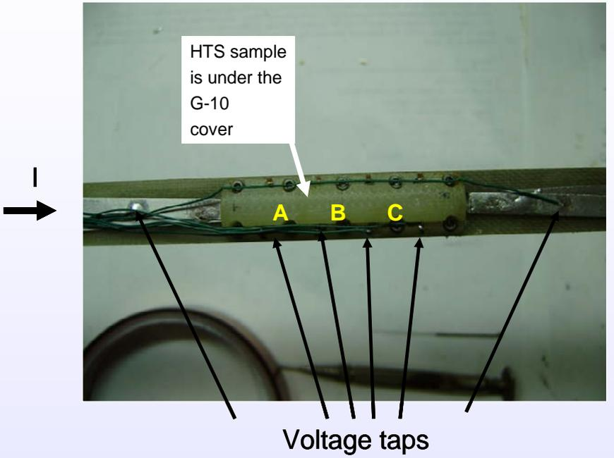
Field is measured with respect to c-axis (see below on right)
