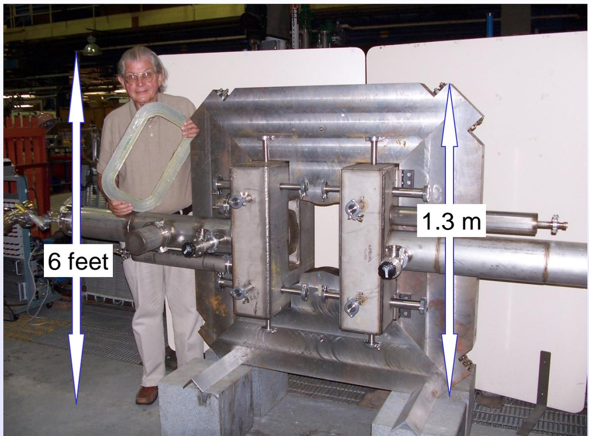
**LN<sub>2</sub> (77 K) Test of Coils Made with ASC 1<sup>st</sup> Generation HTS**
