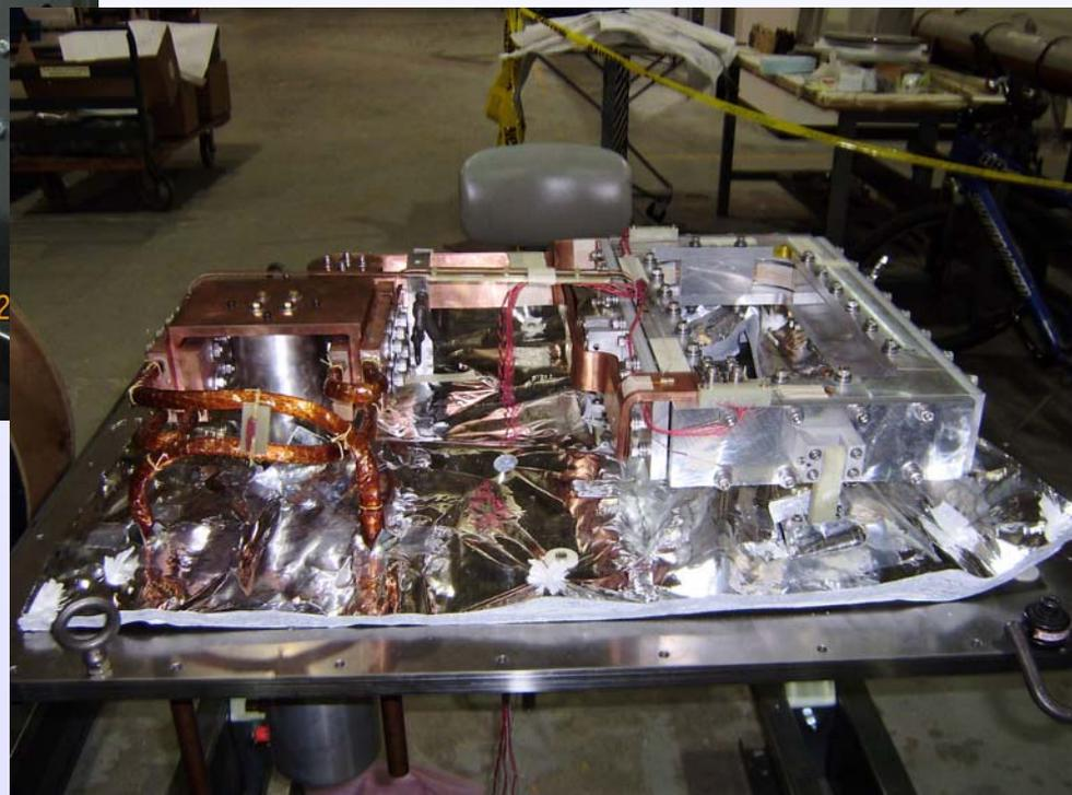
**Coils previously made under separate R&D funding are ready for testing with cryo-coolers**
