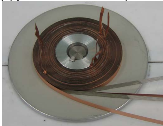
Fig. 7. Small test coil for future R&D. Above is a photo of a bi-filar coil that produces a zero net field and will be used in to study axial compression. Standard pancake coils have also been made for quench protection studies.
