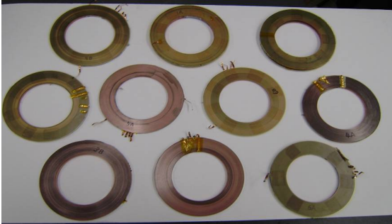
Fig. 2(a) Photograph of single coils: Fourteen single coils were wound and tested in LN 2 . Voltage taps are attached every 50 turns. No indication of local defect was observed in their V-I curves.
