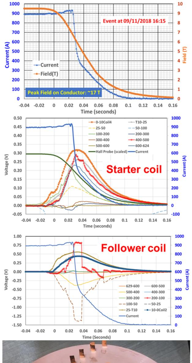
Fig. 9. Thermal runaway (quench) at 4 K in the IBS double-pancake coil. Plot at the top shows how rapidly the field drops, and the middle two plots show how rapidly the quench propagates within each pancake and pancake-to-pancake as measured by voltage taps within the coil (bottom).
