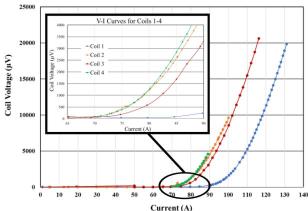
Fig. 6. V-I curves of four single pancake coils tested at 77 K.
