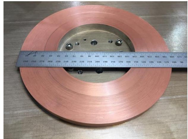
Fig. 3. A single pancake coil with an i.d. of 105 mm and o.d. of 200 mm.
