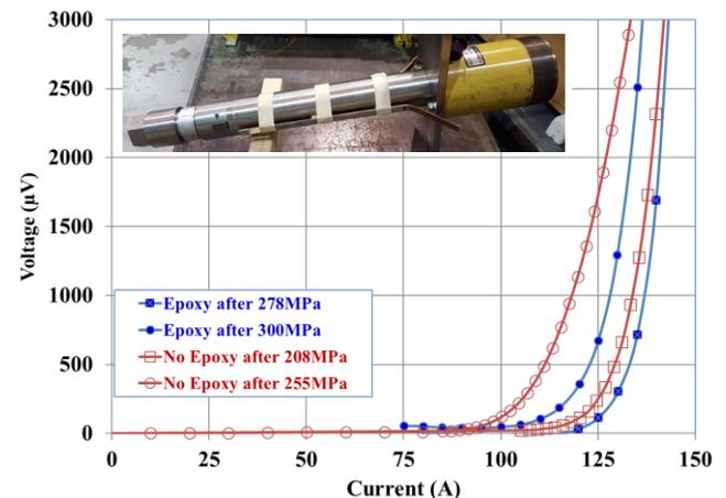
Fig. 4. Influence of loading on the narrow face of HTS tape with 40  $\mu\text{m}$  copper and 50  $\mu\text{m}$  Hastelloy with and without epoxy painted on the surface. A picture of part of the fixture is shown in the inset.
