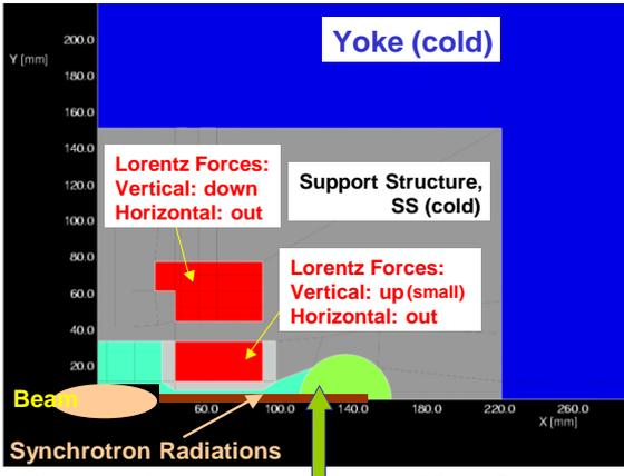
**Synchrotron radiations deposit energy in a warm absorber, that is inside the cryostat. Heat is removed efficiently at higher temperature.**
