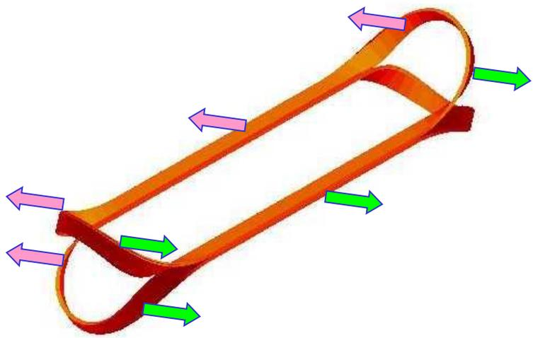
In common coil design, the coil moves as a whole, without straining the conductor in the ends. This is particularly important in high field magnets where forces are large and this may minimize quench or damage.
