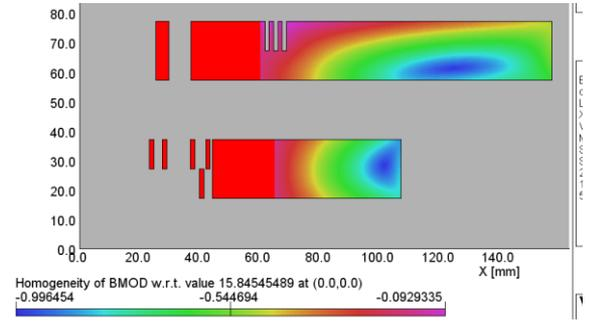
Quench Field: ~16 T with  $J_c = 3000 \text{ A/mm}^2$ , Cu/Non-cu = 0.85
