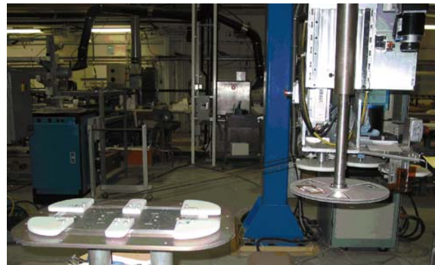
Figure 1: A coil being wound on the new computer controlled winding machine.
