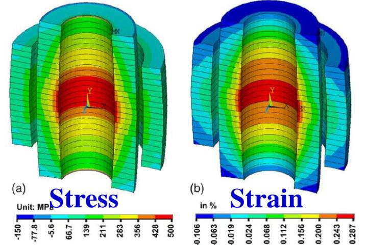
S.L. Lalitha and R.C. Gupta, "The Mechanical Design Optimization of a High Field HTS Solenoid" @ASC2014
