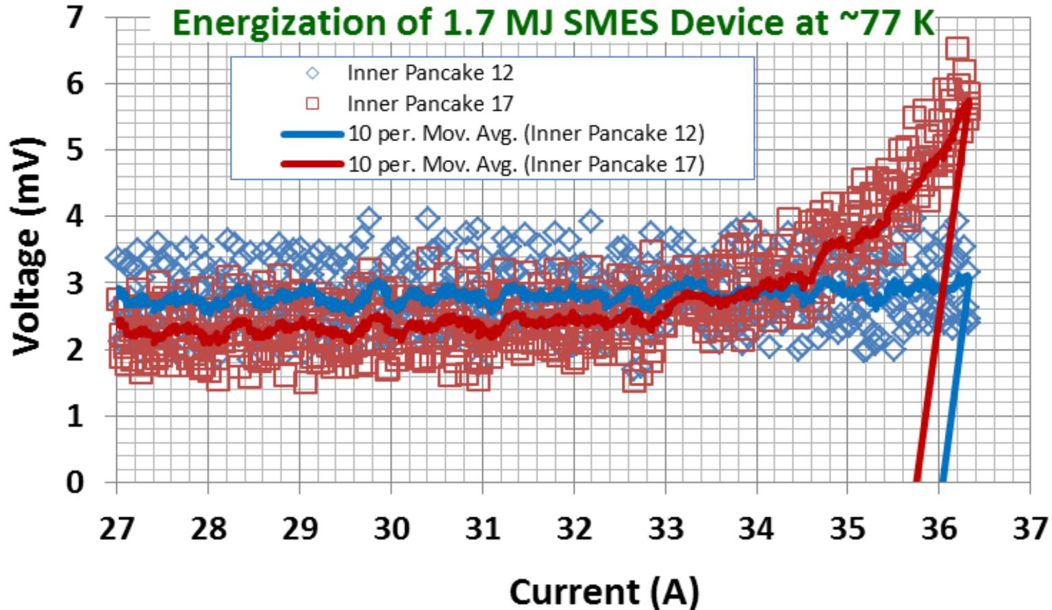
**Power supply was shut off and energy extracted when the quench threshold reached. No degradation in coil performance observed**
