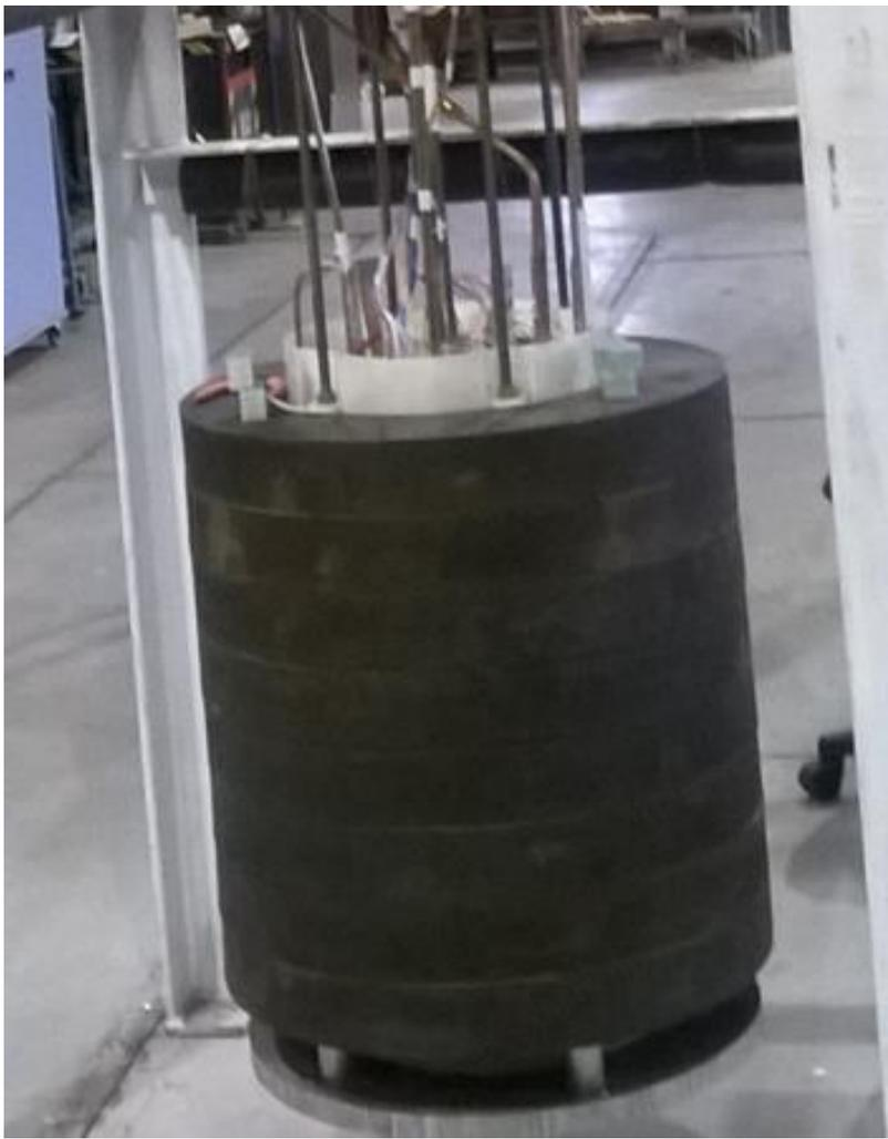
**Outer inserted over inner coil**
