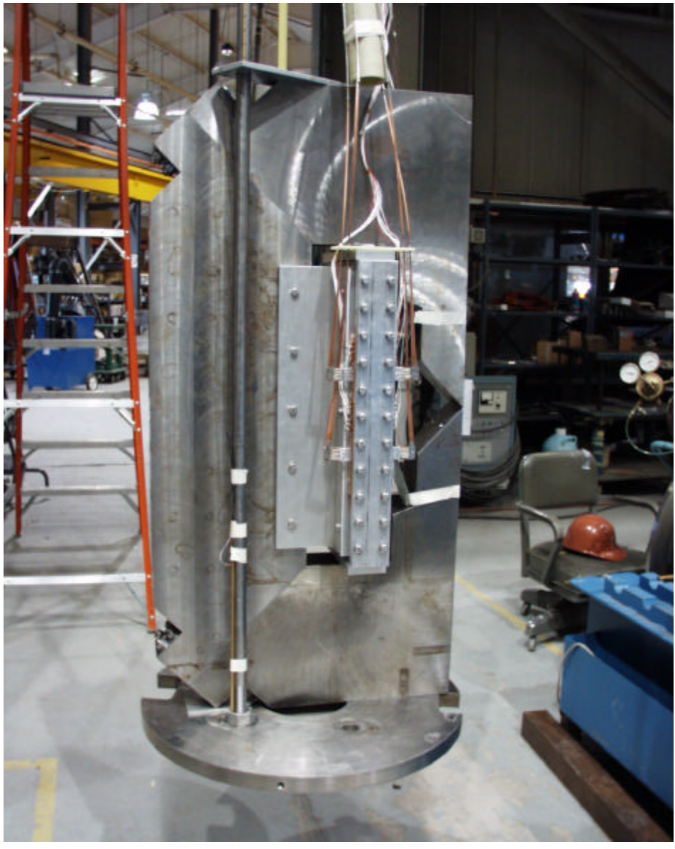
Magnetic mirror model magnet, just before the test. At the test facility, the magnet can be tested in a wide range of temperature (4.2 K to 80 K). A higher operating temperature translates in to a significant reduction in operating cost.
