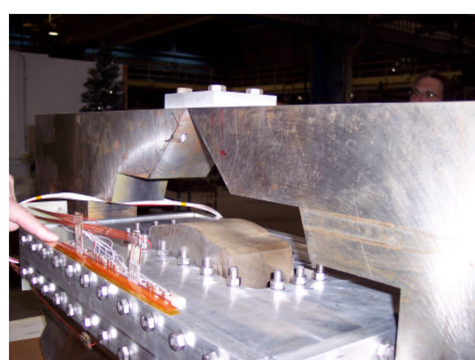
Coils in their bolted support structure, with the pole iron (in the middle, inside the structure), magnetic mirrors (two on the upper side with 45 degree angles on either side of the vertical axis) and iron return yoke.
