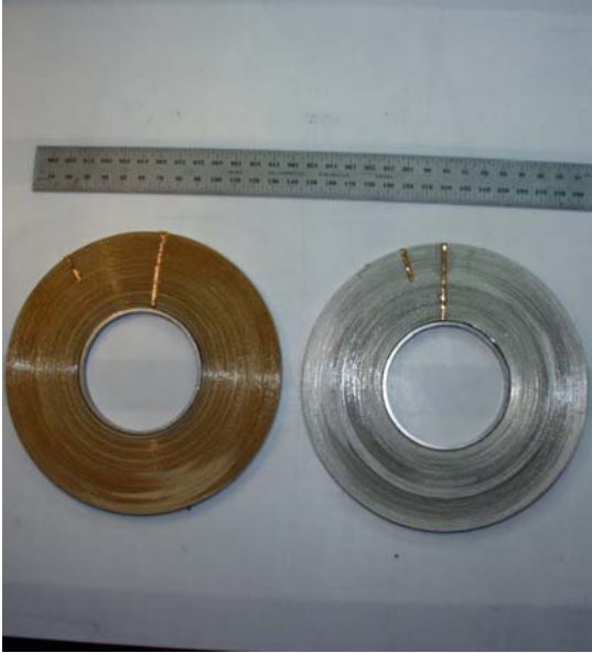
Fig. 2: Two double pancake NMR coils, with conventional kapton insulation on left and stainless steel tape insulation on right.
