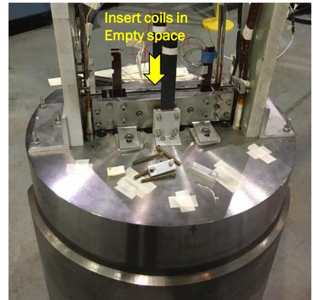
HTS coils inside Nb<sub>3</sub>Sn dipole - early experience of HTS/LTS hybrid dipole
