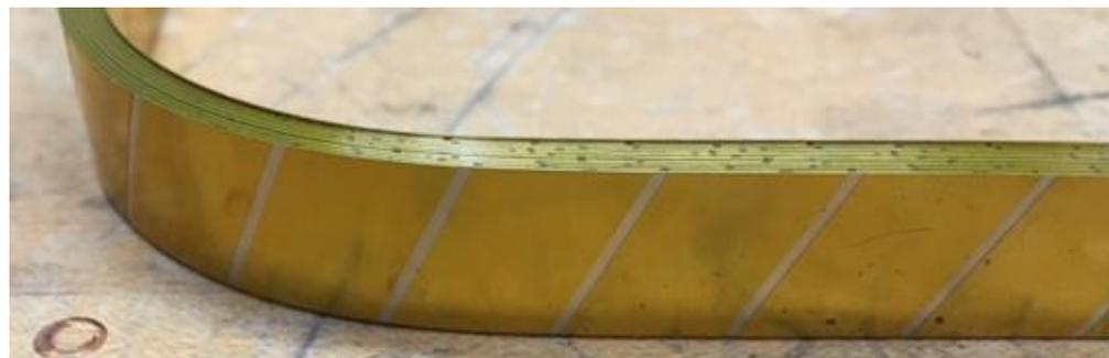
77 K tests show no degradation in conductor performance
