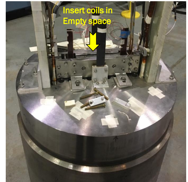
HTS coils inside Nb 3 Sn dipole - early experience of HTS/LTS hybrid dipole
