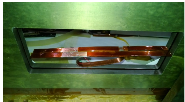
Fig. 4. A flexible HTS splice with copper stabilizer allowing a small relative motion of a few mm. The splice resides in the low field region of the BNL Nb 3 Sn common coil dipole DCC017.
