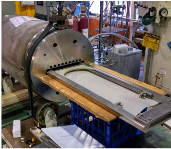
Fig. 1. A magnet wherein new coils in a fixture can be inserted in the magnet without any need to disassemble and reassemble the magnet (coils are not included in the fixture above).
