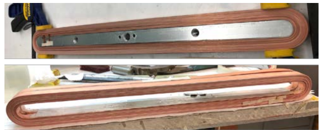
Fig. 10. One HTS single-pancake (top) and two single-pancakes spliced as a double-pancake (bottom) coil in preparation for testing with the BNL \text{Nb}_3\text{Sn} common coil dipole DCC017 to provide a background field of \sim 10 T.
