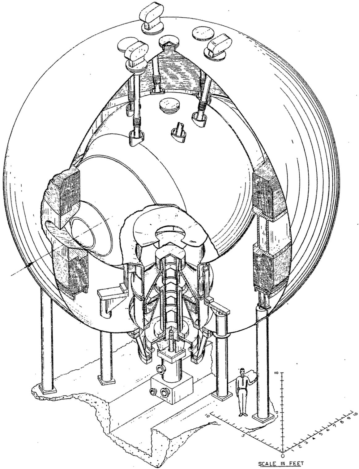
Fig. 6. 25-ft bubble chamber main assembly - isometric view.
