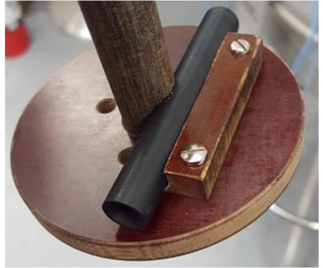
Fig. 3. Bi2223 tube provided by CAN superconductor [10]. The tube and tube holder will be inserted inside the bore of a coil providing background field.
