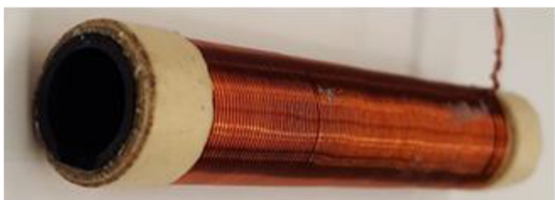
Fig. 5. Copper windings on the HTS tube to immerse it in a field that is primarily axial.
