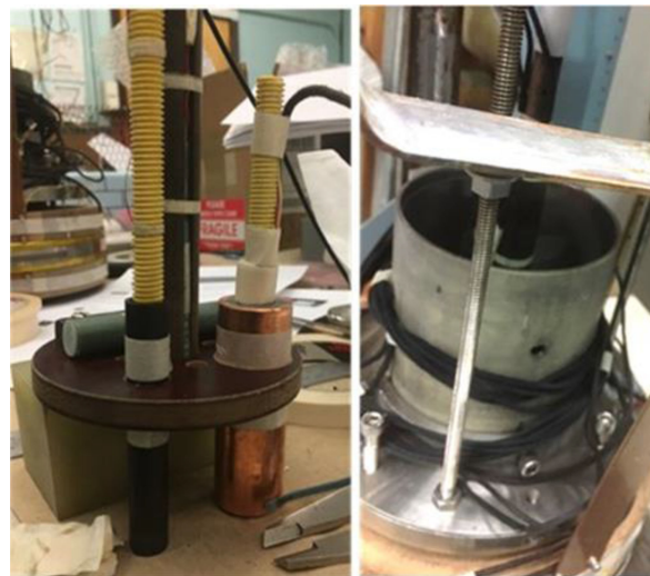
Fig. 8. Left: Disc with tubes of HTS (black) and LTS (copper-clad NbTi), and a center tube holding a Hall probe on the axis of the disc. Right: The disc, with three Hall probes, inside the superconducting coil for testing at 4 K.
