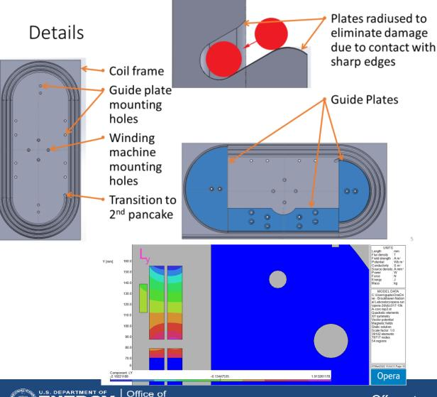
Net vertical force (density) is insert CORC coil downward. The peak is smaller than that in  $Nb_3Sn$  coils. However, the turns are captured in a structure. Moreover, the bobbin can take the net downward forces.
