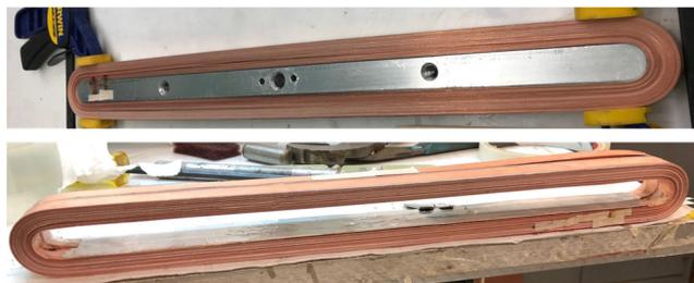
Fig. 10. One HTS single-pancake (top) and two single-pancakes spliced as a double-pancake (bottom) coil in preparation for testing with the BNL  $Nb_3Sn$  common coil dipole DCC017 to provide a background field of  $\sim 10$  T.
