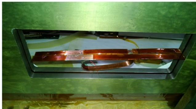
Fig. 4. A flexible HTS splice with copper stabilizer allowing a small relative motion of a few mm. The splice resides in the low field region of the BNL Nb<sub>3</sub>Sn common coil dipole DCC017.
