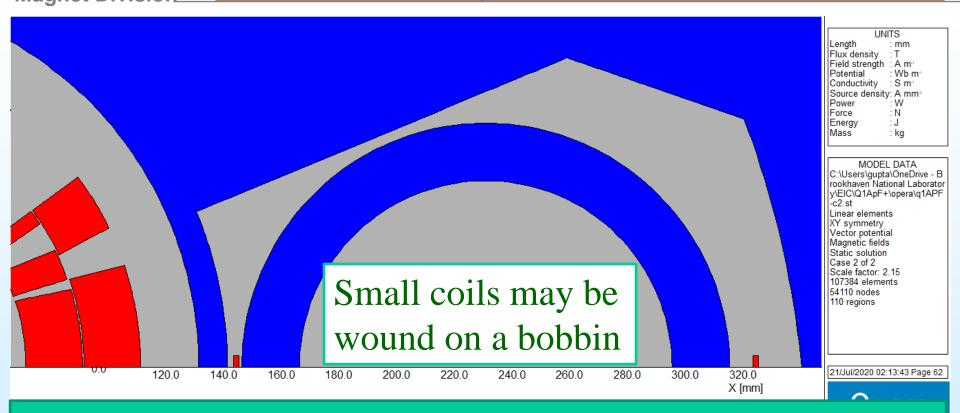
Path of flux lines navigated with cutout in yoke and small coils on the two side of yoke over e-beam region added to further navigate flux lines (and reduce saturation) to significantly reduce field in the e-beam region
