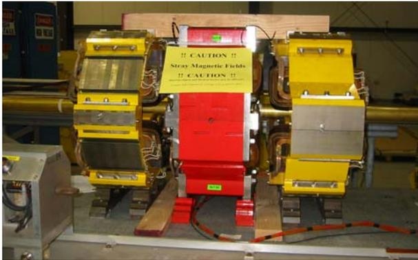
Figure 10: SLS Quadrupole and sextupole on the measuring stand to study interaction harmonics between the magnets.
