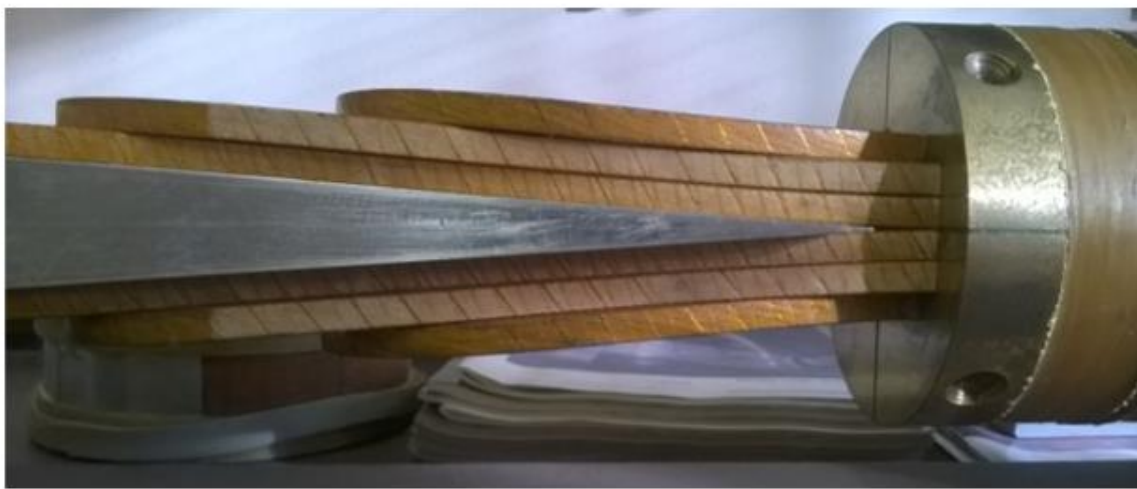
Figure 2: Nb 3 Sn block coil dipole with cross-section (left) and lifted ends (right).
