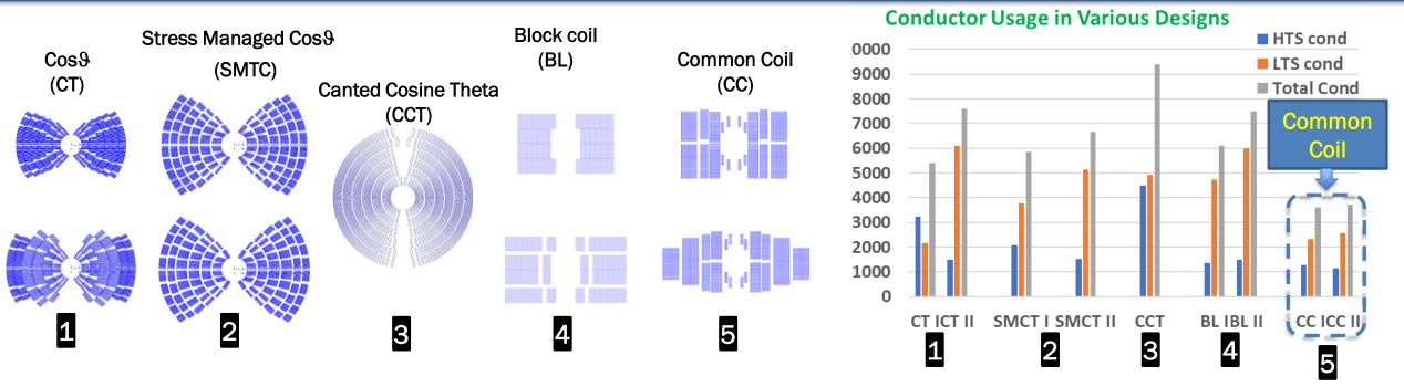
Comparative studies of 20 T designs (as presented at MT) revealed that the common coil design uses significantly less conductor (including less HTS) than the other designs. This was a surprise initially; now understood and validated.
