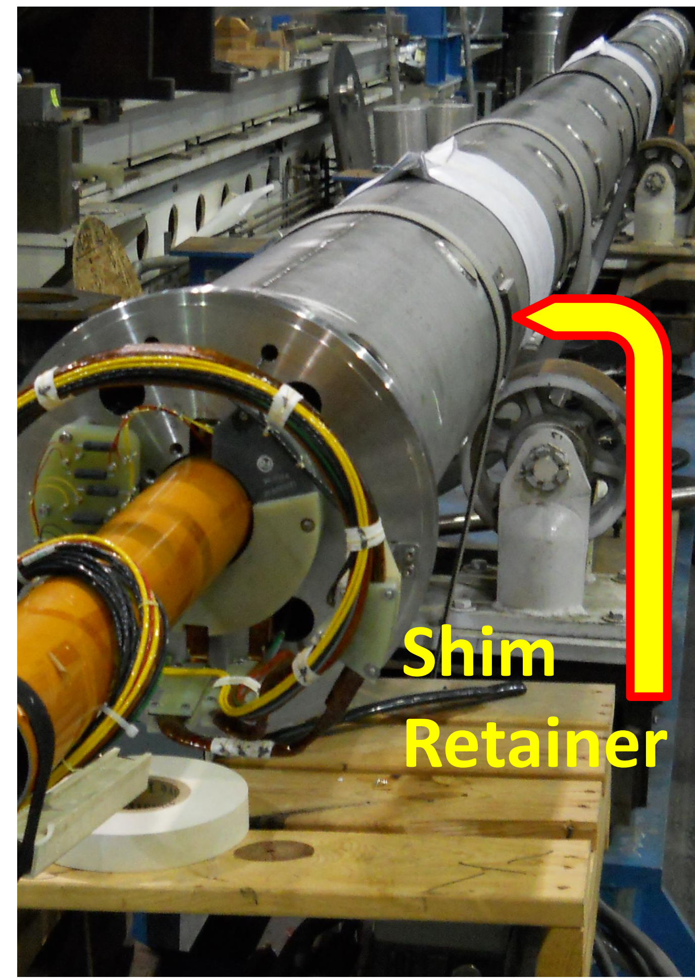
Magnetic model of the D1 magnet with the Iron Shim indicated and the actual magnet during the construction (shims will be placed in the Shim Retainer).
