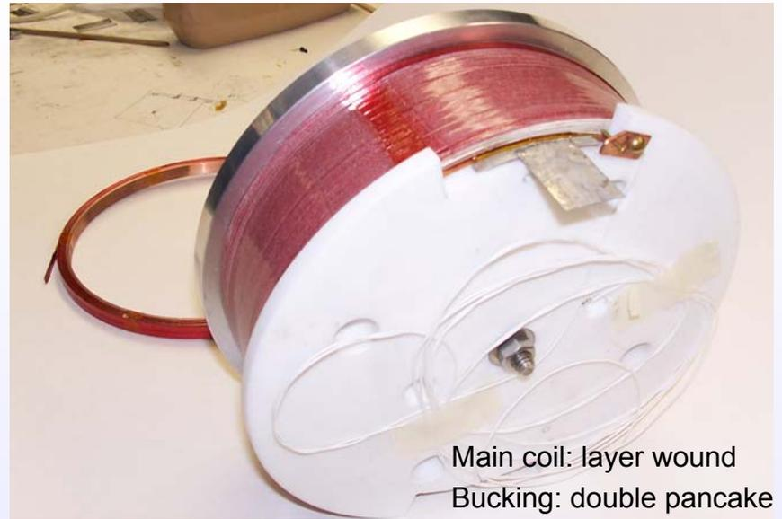
Well above design current is obtained @77 K in the liquid nitrogen testing itself.
