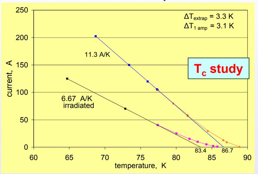
**Bottom line – YBCO is robust against radiation damage:**
