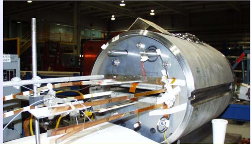
**Record 10.4 T in R&W Nb<sub>3</sub>Sn Magnet**
