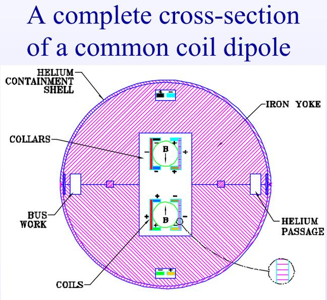
Magnets based on this design have been built at LBL and Fermilab also.
