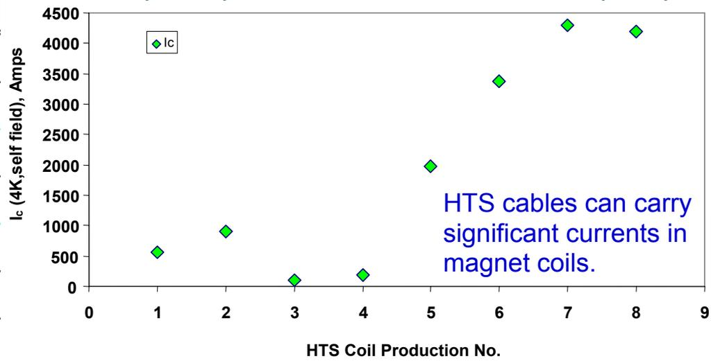
**Early demonstration that HTS coils with high current Rutherford cable can be built and they can be used in a design that is suitable for collider dipole.**
