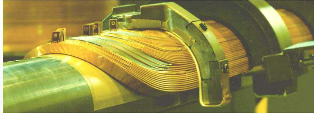
RHIC dipole with complex 3-d geometry in the ends
