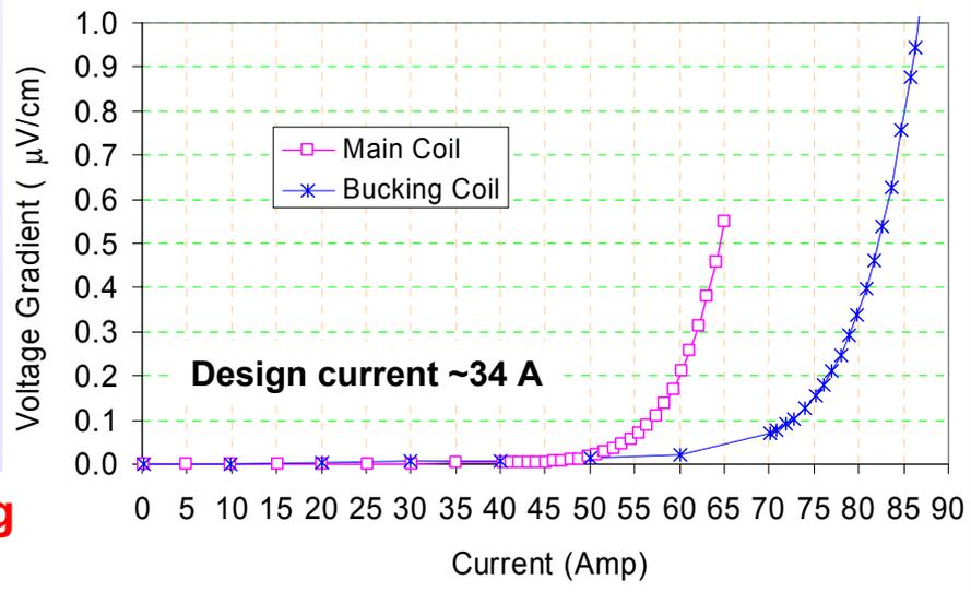
Nitrogen testing at 77 K rather than Helium testing at 4 K for NbTi provided a significant savings.
