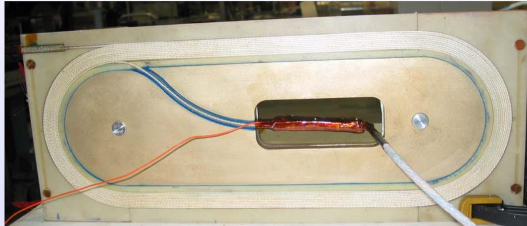
Racetrack HTS coil for common coil design
