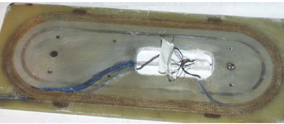
HTS cable coil prior to vacuum impregnation
