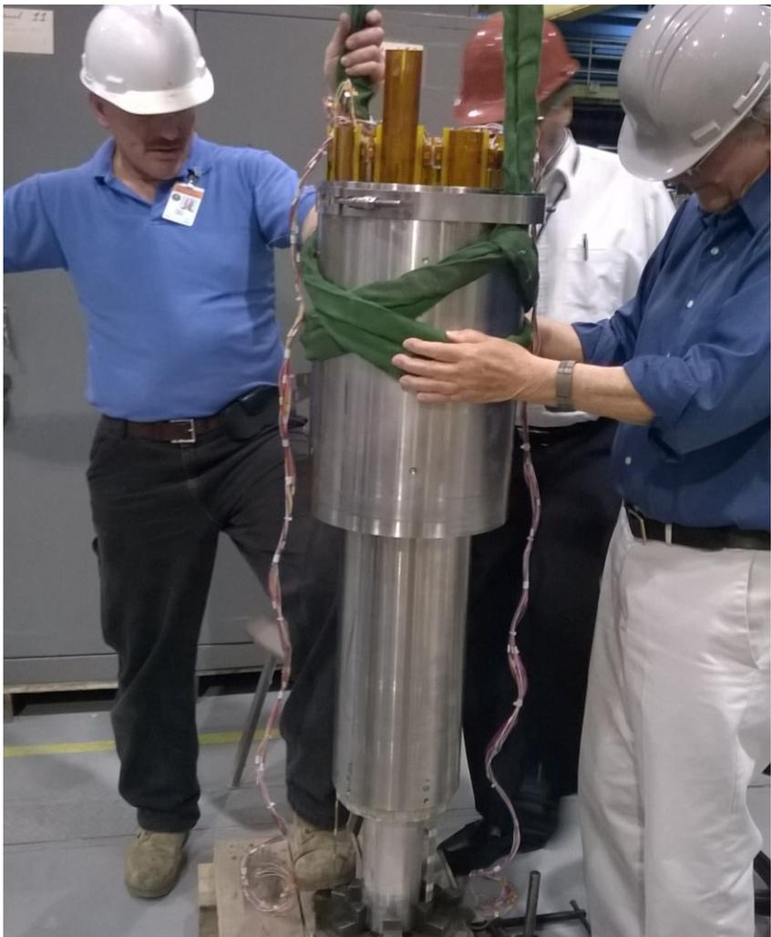
**Outer inserted over inner coil**
