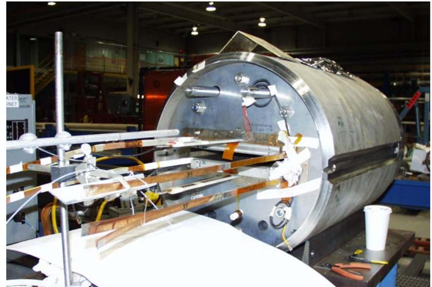
HTS insert coil test configuration
