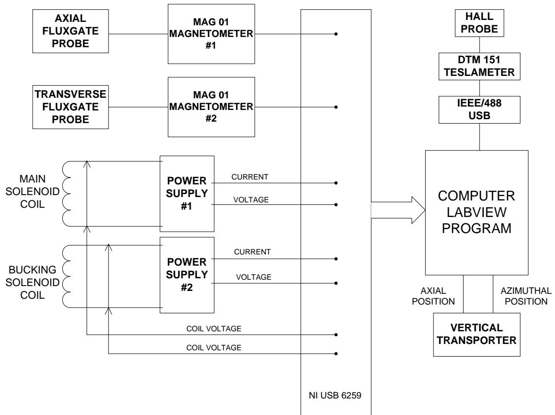
Fig. 3.7. Block Diagram of Measurement and Data Acquisition System
