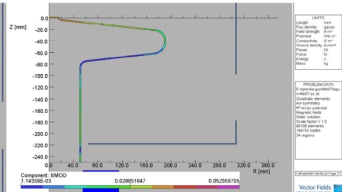
Fig. 1.8. Field (in Gauss) on the surface of superconducting cavity based on a model superconducting shield with the bucking solenoid turned on at the nominal current (left) and turned off (right). One can clearly see a reduction. However, given the sensitive nature of these calculations, magnetic measurements are planned at  $\sim 77\text{ K}$ .
