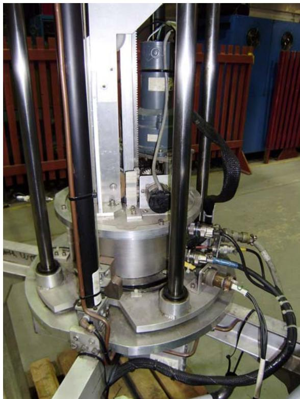
*Figure 3.2. Close up vertical transporter drive mechanisms.*
