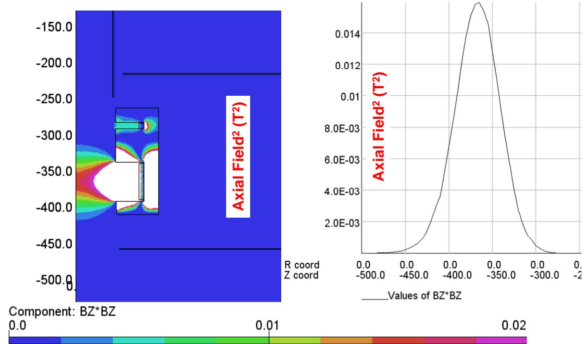
Fig. 1.4. Computed map of the focusing ( $B_z^2$ ) is shown on the left and the axial profile of the focusing ( $B_z^2$ ) along the beam axis is shown on the right. Beam is injected in the cavity at  $z=0$  and travels downward (negative  $z$ ).
