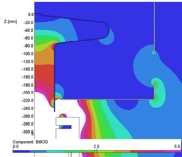
Fig. 1.7. Field map (in Gauss) with the bucking solenoid turned on at the nominal current (left) and turned off (right). One can clearly see the reduction in field inside the cavity. One can also see the reduction in leakage field on the cavity and inside the inner magnetic shield.
