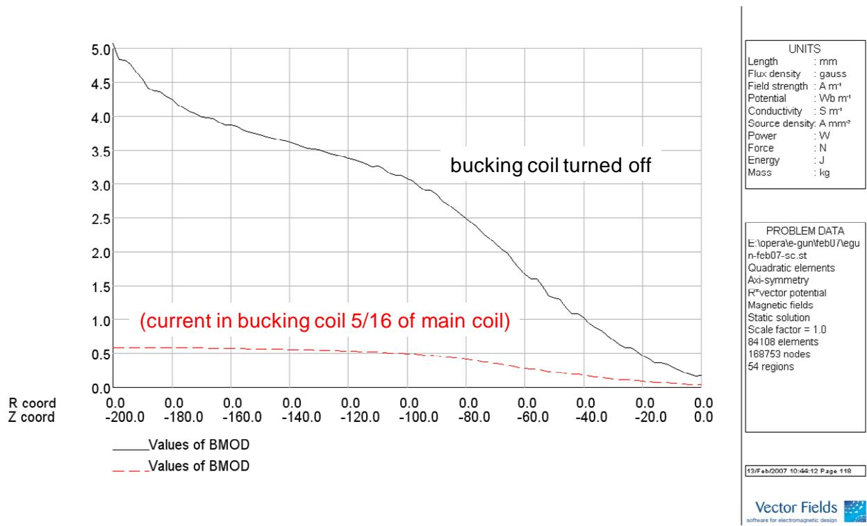
Fig.1.5. Magnitude of the field inside the axis of cavity with and without bucking coil. Current in the bucking coil can be adjusted to further minimize the field at the center or at the surface of the cavity.
