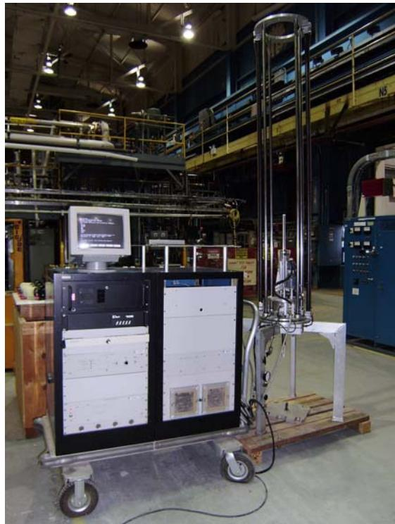
*Figure 3.1. Vertical transporter and computer control cart.*
