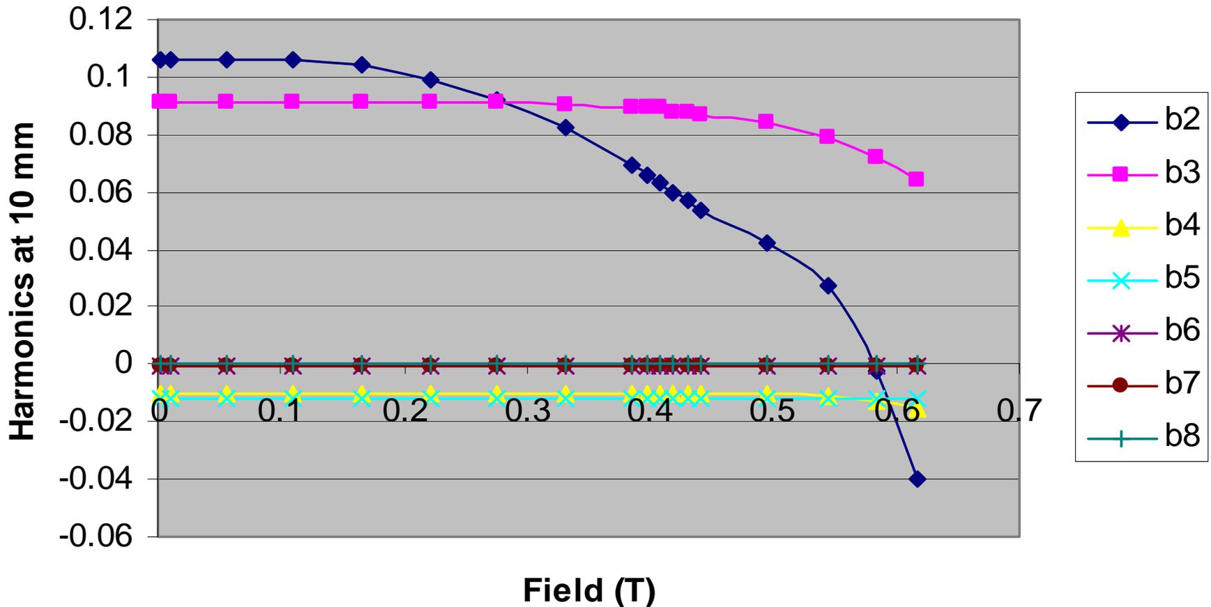
**Note: Small values of field harmonics (only a few parts in  $10^5$  even at 20 mm radius).**
