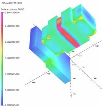
Put shield on both sides for symmetry. Would need to adjust iron in two outside poles of 3-pole wiggler to maintain zero integral.
