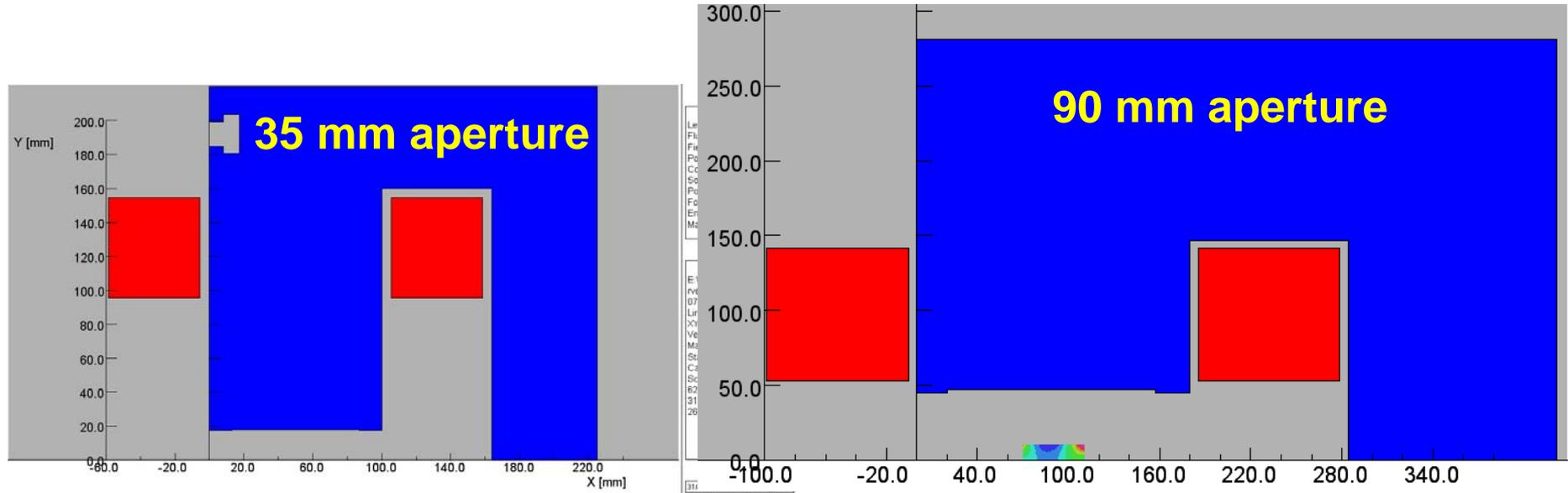
Note: 90 mm is the minimum vertical clearance. Pole gap at the magnet center is higher. Adjust number of turns and then pole gap of 90 mm dipole to match transfer function with 35 mm aperture dipole to allow the same power supply for both magnets.
