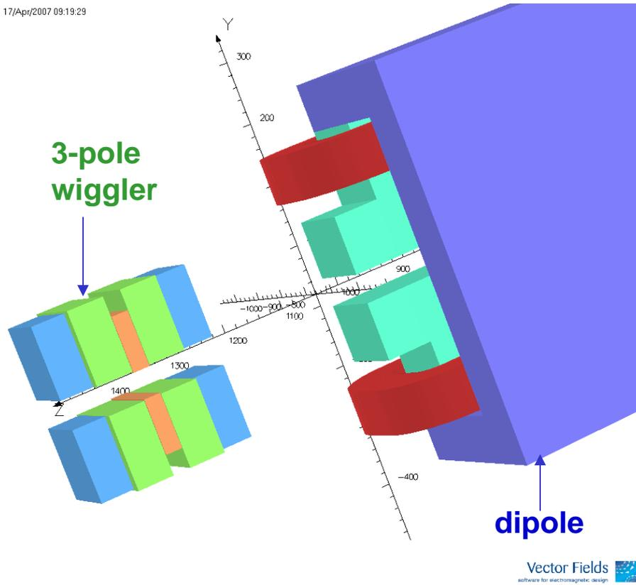
This design allows racetrack coils and ~18 cm of free space between dipole and 3pole wiggler.
