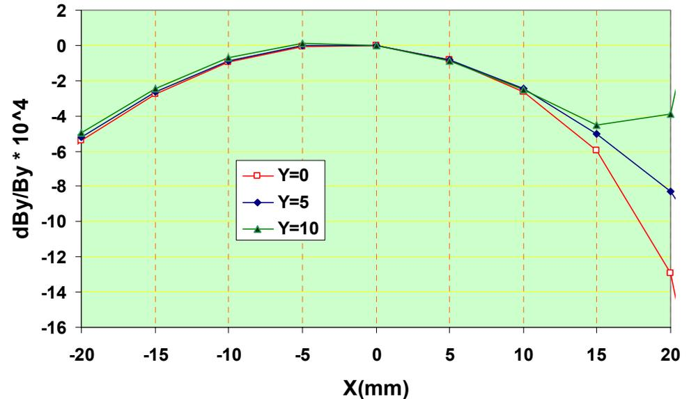
As per plan, the nose will be chamfered to minimize the measured integrated error. Field quality specs are expected to be met.
