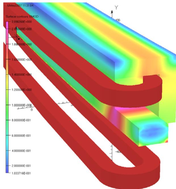
However, if the relative drop is due to iron saturation, then the drop would be lower at lower fields (lower saturation, as here).
