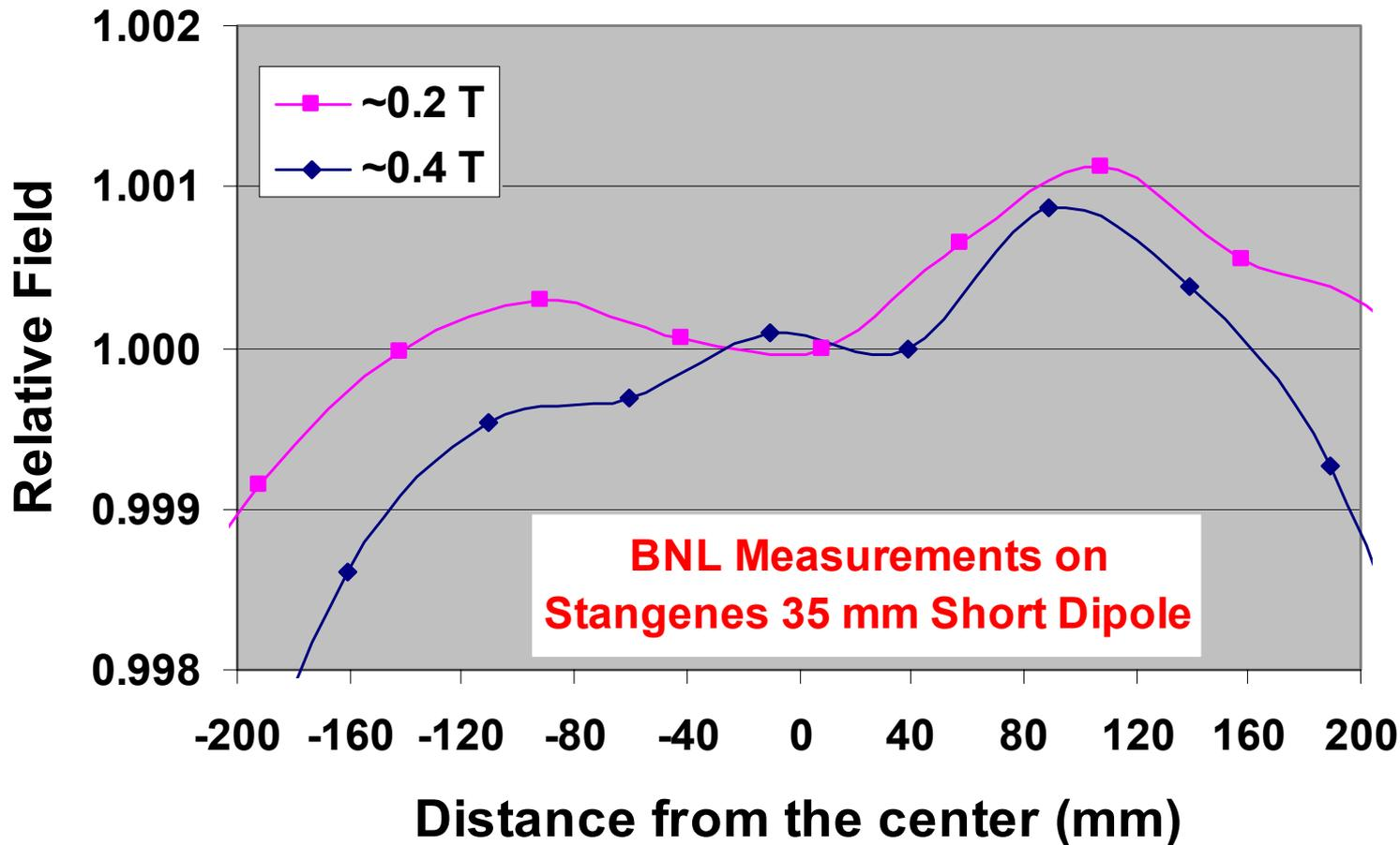
**A few part in 1,000 variation has been observed along the magnet length. Possible cause (mechanical or magnetic) is under investigation.**
