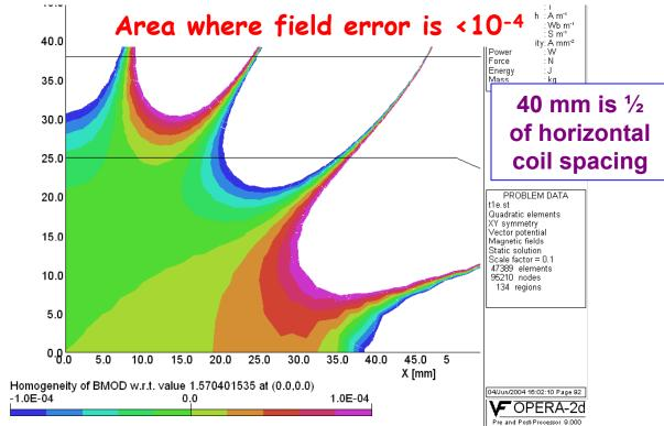
Field errors should be minimized for actual beam trajectory & beam size. It was sort of done when the design concept was being optimized by hand. Optimization programs are being modified to include various scenarios. Waiting for feed back from Beam Physicists on how best to optimize. However, the design as such looks good and should be adequate.
