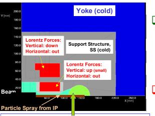
A large amount of particles coming from high luminosity IP deposit energy in a warm (or 80 K) absorber, that is inside the cryostat. Heat is removed efficiently at higher temperature.
