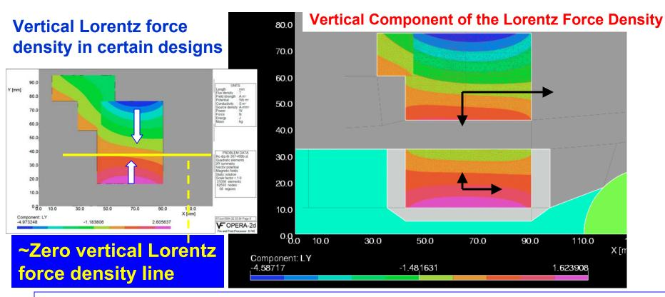
Since there is no downward force on the lower block (there is slight upward force), we do not need much support below it, if the structure is segmented. The support structure can be designed to deal with the downward force on the upper block using the space between the upper and the lower blocks.
