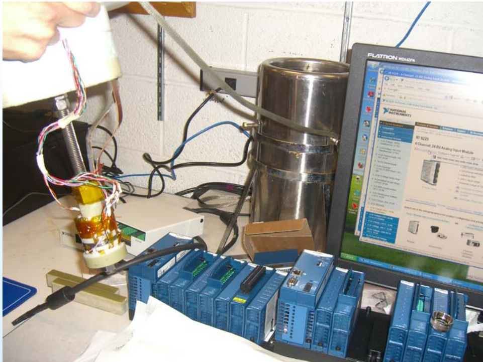
Small coils: ~10 meter tape (we can afford to sacrifice them to understand the limit)
