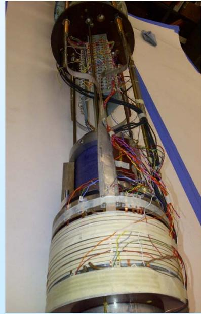
*Coil could have reached above 10 T peak (original target), but was not ramped up to protect electronics of that time. Full solenoid with 24 pancakes should create >10 T on axis.*
