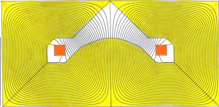
*Cold iron magnetic mirror model with six coils in a bolted support structure.*
