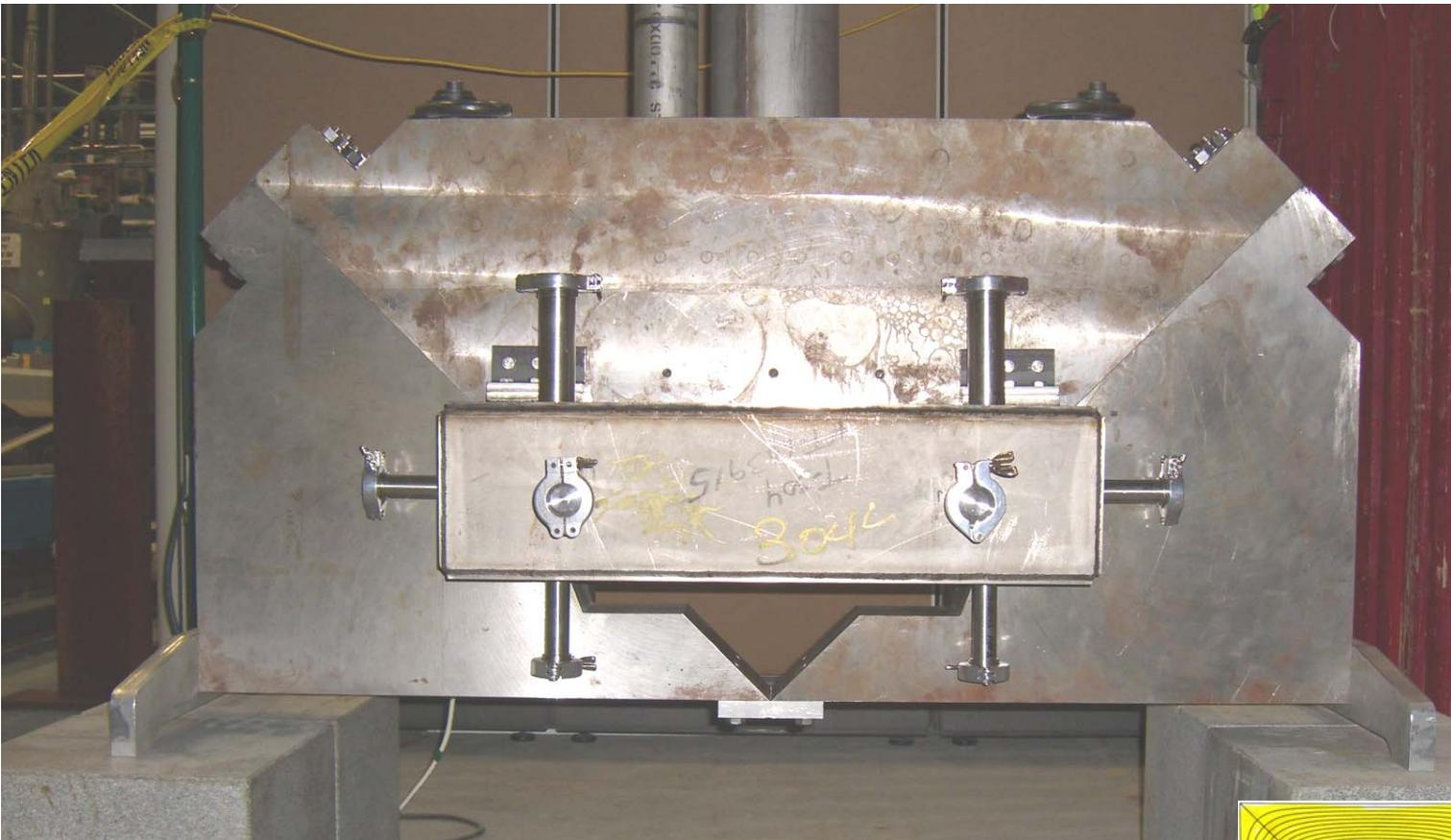
**Warm iron magnetic mirror model with twelve coils in its own cryostat**
