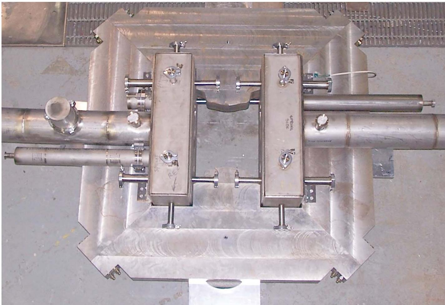
**Warm iron quadrupole with twenty four coils in two cryostats**
