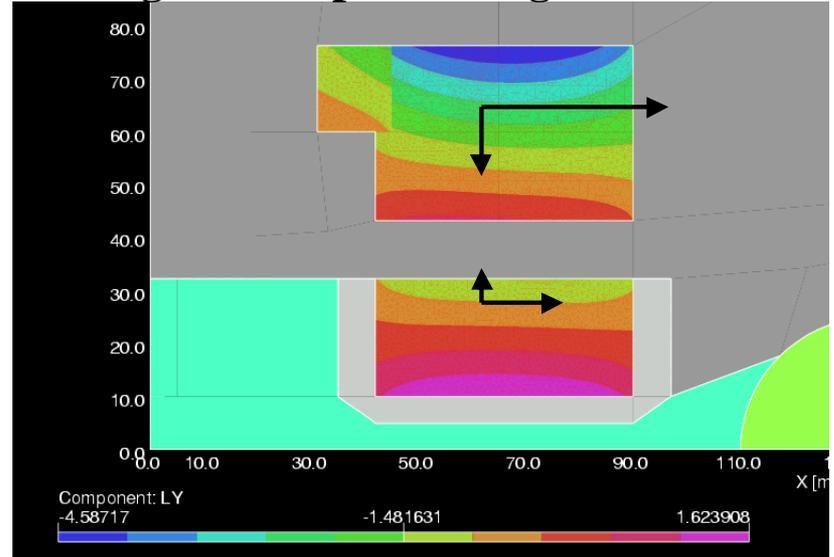
Since there is no downward force on the lower block (there is slight upward force), we do not need much support below if the structure is segmented. The support structure can be designed to deal with the downward force on the upper block using the space between the upper and the lower blocks.
