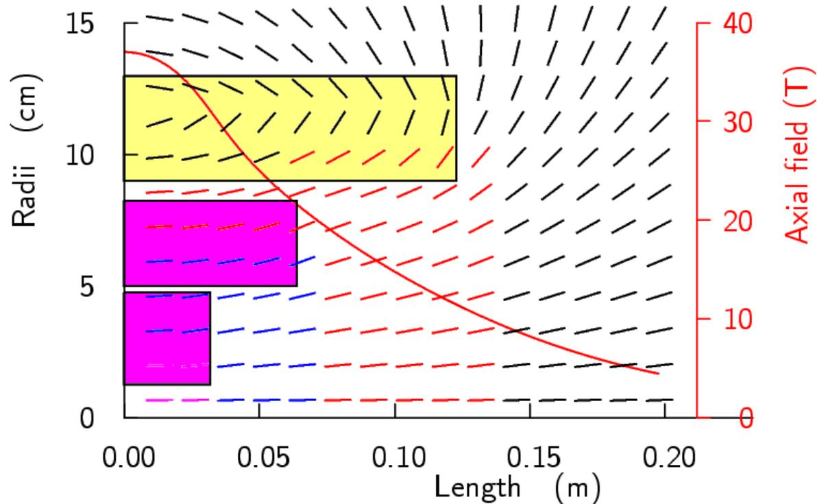
Field directions and axial fields for the combined magnet using
