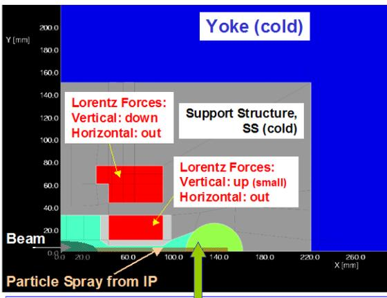
A large amount of particles coming from high luminosity IP deposit energy in a warm (or 80 K) absorber, that is inside the cryostat. Heat is removed efficiently at higher temperature.
