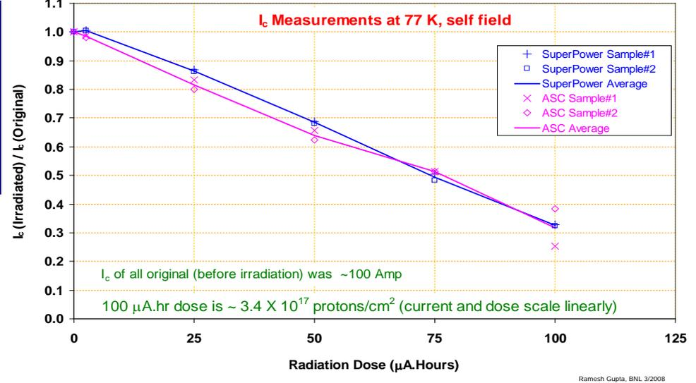
One needs to normalize the impact of this damage for muon collider magnets
