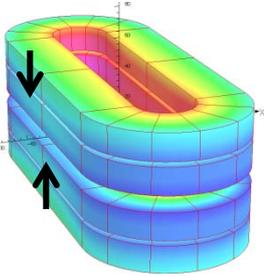
In conventional designs the upper and lower coils rest (react) against each other. In a truly open midplane design, the target is to have no structure between upper and lower coils. Structure generates large heat loads and the goal is to minimize them.
