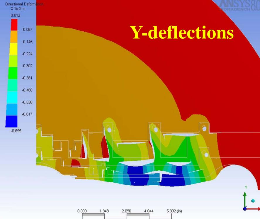
**In the present design the relative values of the x and y deflections are 3-4 mil (100 micron) and the maximum value is 6-7 mil (170 micron).**
