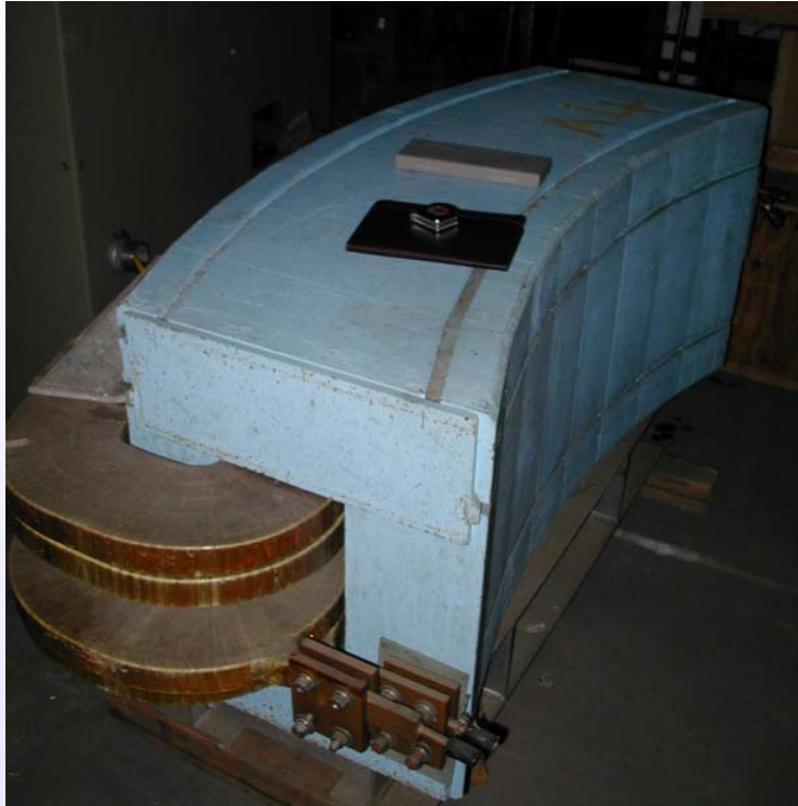
Magnet in the existing NSLS complex (a typical design for iron dominated magnets)
