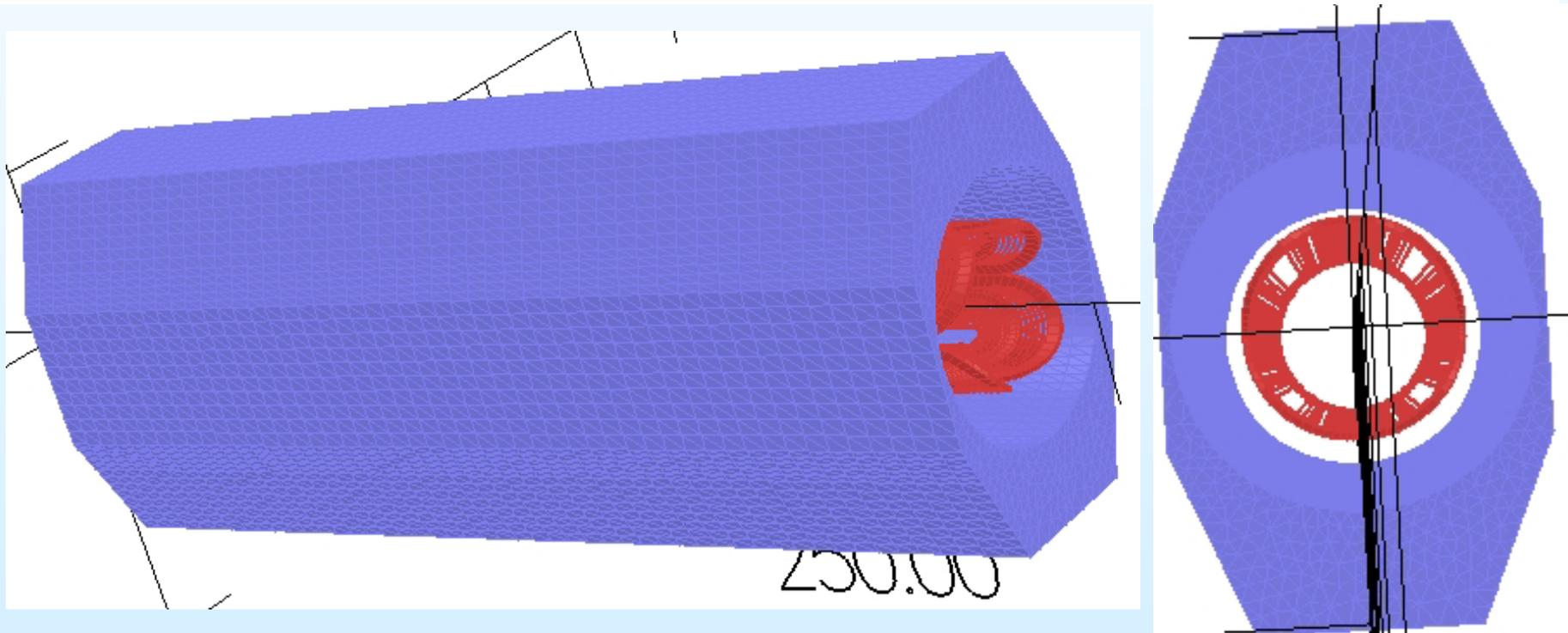
Need only  $\frac{1}{2}$  of this model for calculations. Apply boundary conditions on right and left side to simulate various cases. Need only  $\frac{1}{4}$  of the model if boundary condition is the same on the left and right side.
