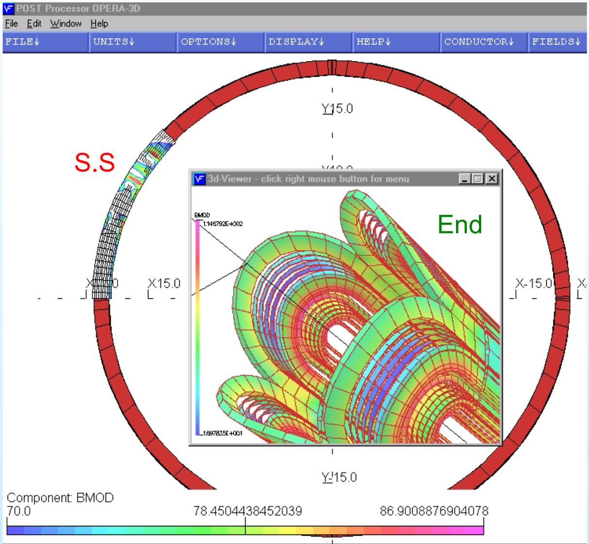
Based on the preliminary calculations, the peak value in Design A is larger in the end. The peak field in the end will be minimized more in Design B.
