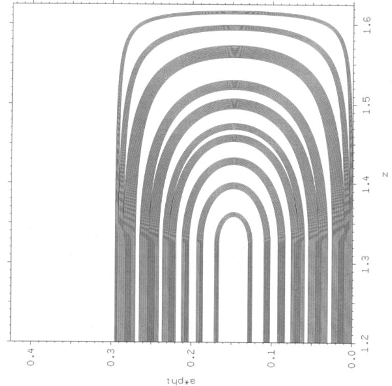
Fig. 4. End-turn layout on the developed winding cylinder with the shape function of Fig. 1, the 2-D design of Table II, and the block group definition of Table II, showing individual turns.
