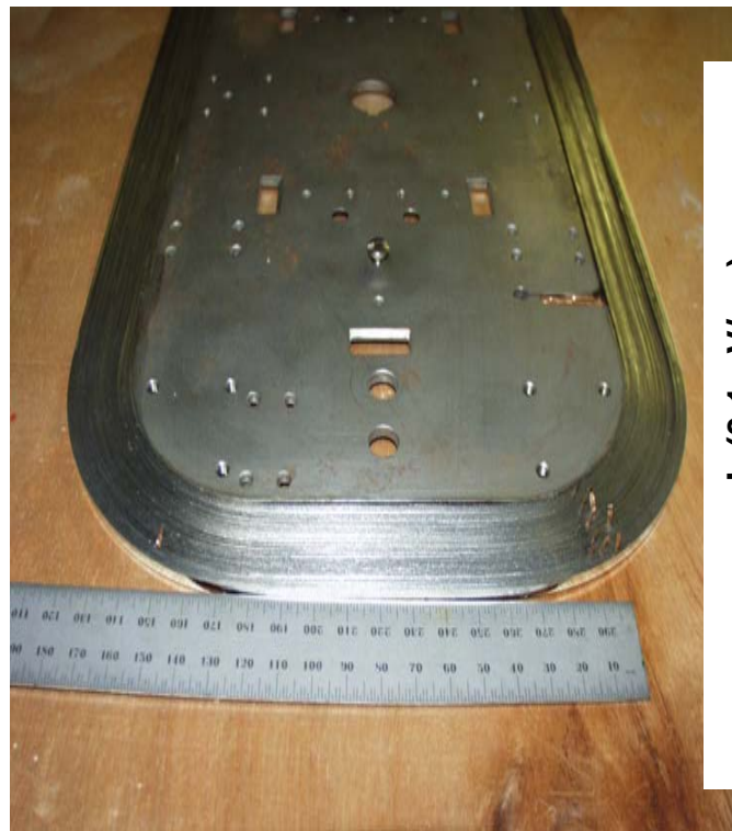
Coil made with YBCO
