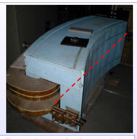
In the proposed design the HTS coil will go on the outer lag (return yoke). One side of the coil will be curved and other side will be straight and thus the problem of negative curvature (sagitta) will be avoided.
