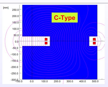
We prefer C-type over H-type. It should produce lower cost HTS magnets
