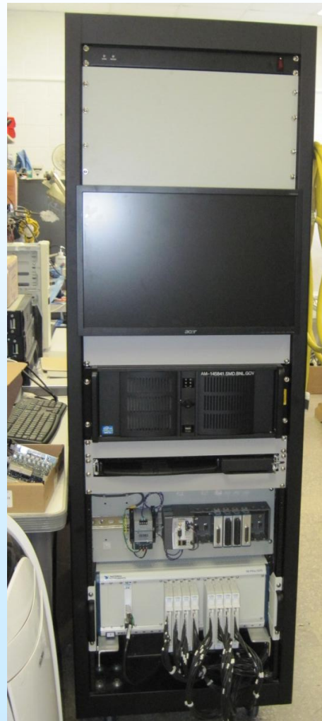
Cabinet #2 (32 channels, 1kV) (expandable to 64 and 3kV)
