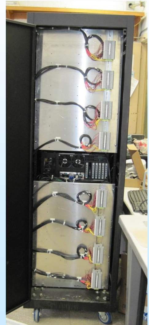
Cabinet #2 (32 channels, 1kV) (expandable to 64 and 3kV)
