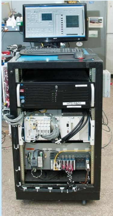
Cabinet #1 (32 channels, 1kV)
