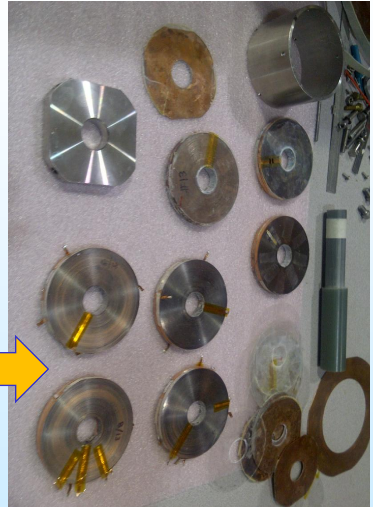
HTS insert taken apart with a few parts displayed
