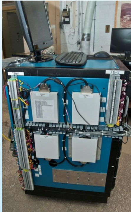
Cabinet #1 (32 channels, 1kV)
