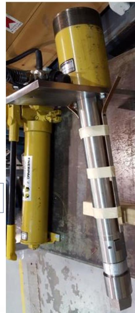
ENERPAC RCH-302 Hollow Plunger Cylinder
